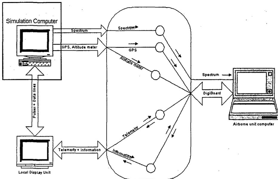
Figure.4 - Schematic description of the system
