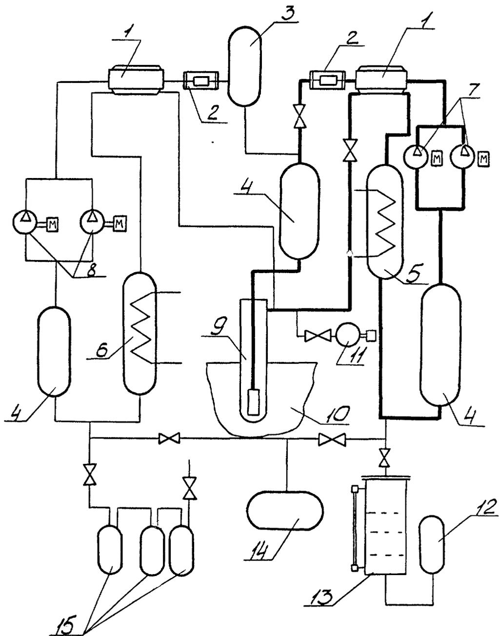
Fig 2. Principle scheme of a gas-cooled loop plant working on dissociating  $N_2O_4$  coolant for investigation of fuel element workability.
