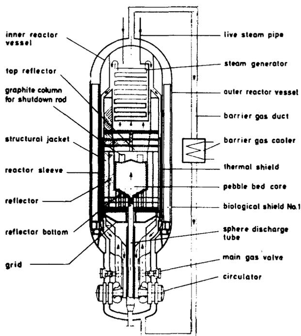
Fig. 1: Vertical Cross Section of AVR Reactor
