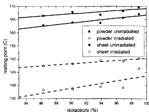
Fig.6.The dependence of melting point on the isotacticity(first scanning, in vacuum).
