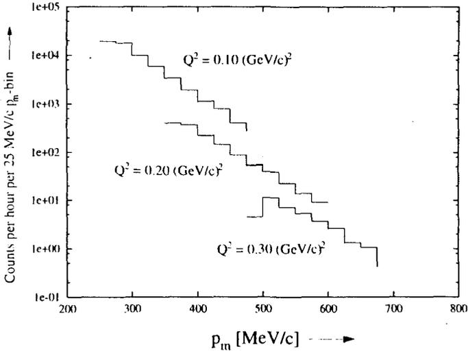
Figure 2: Expected count rate for the  ${}^2\text{H}(e,e'p)$  experiment that was recently performed at the AmPS facility. The calculations assume an average beam current of  $5 \mu\text{A}$ , a target thickness of  $250 \text{ mg/cm}^2$  and the detector solid angles mentioned in the text. The three  $Q^2$ -regions covered by the experiment are indicated.
