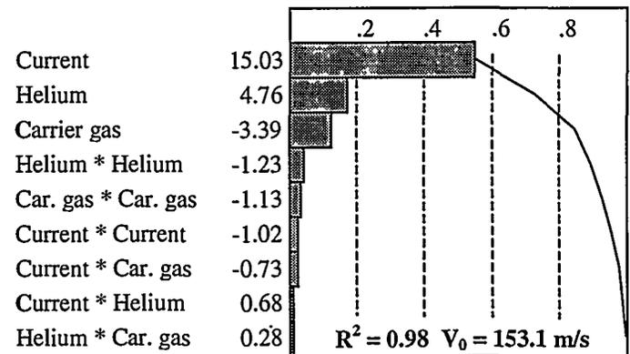
Figure 8. Pareto plot of parameter effects on particle velocity.
