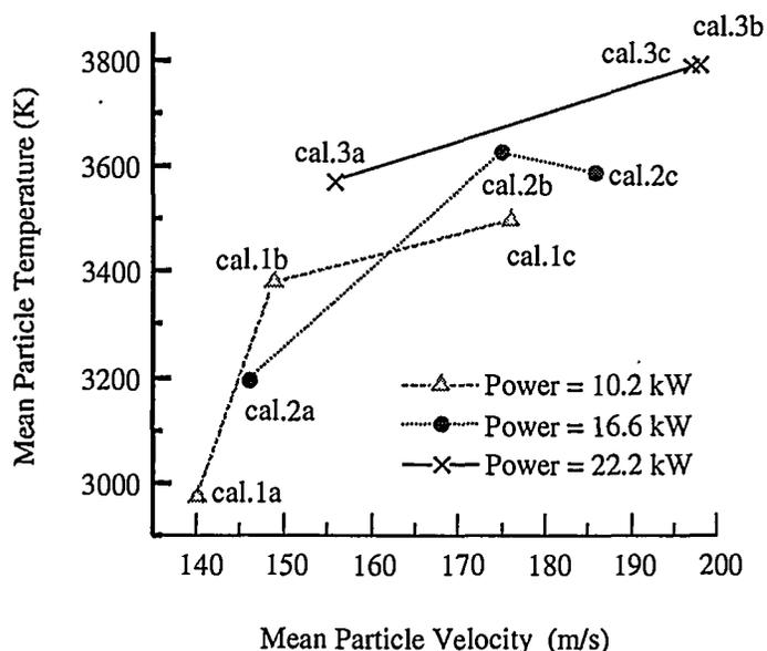
Figure 12. Effect of plasma power and powder injection velocity on in-flight particle temperature and velocity.
