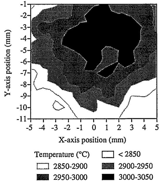
Figure 4. Distribution of particle temperatures within a plume cross-section at 100 mm stand-off and "central" conditions.
