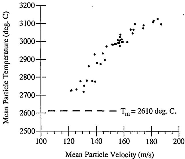
Figure 5. Mean particle temperatures and velocities at the various spray conditions are highly correlated.
