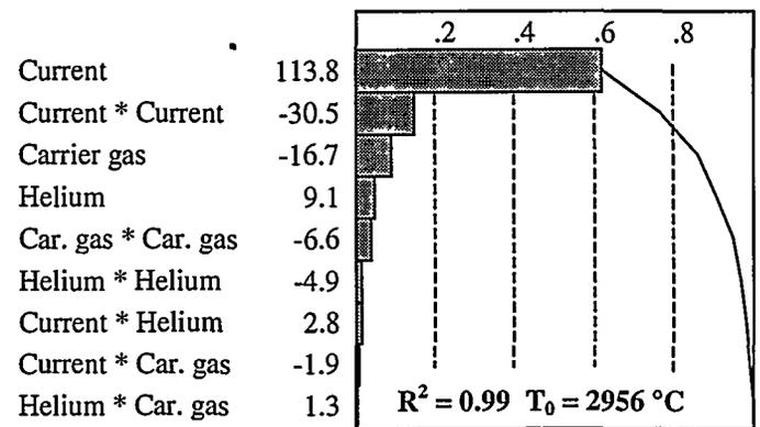
Fig. 7. Pareto plot of parameter effects on particle temperature.
