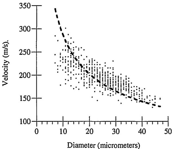
Figure 6. Particle velocities for a given run agree with a simple aerodynamic drag model ( $V \propto 1/d^{1/2}$ ).
