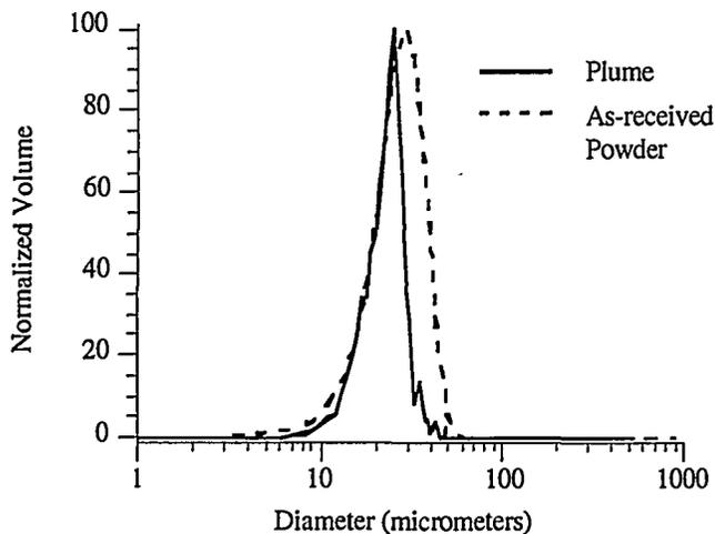
Figure 1. Molybdenum powder size distributions.
