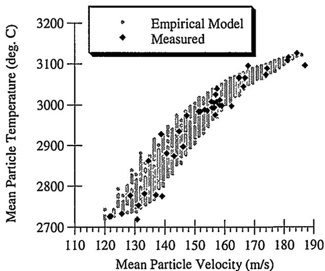
Figure 9. Predicted and measured values for mean particle temperature and velocity.
