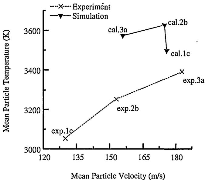
Figure. 10. Computational results for particle injection velocities estimated from carrier gas flow rates.
