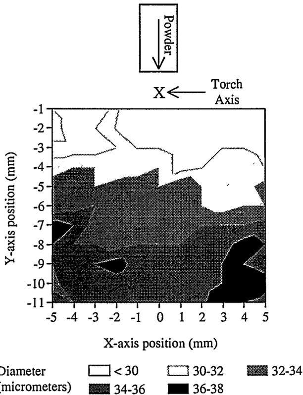
Figure 3. Distribution of particle diameters within a plume cross-section at 100 mm stand-off. Data collected at "central" conditions (700 A, 18 slpm He, 2.0 slpm carrier gas). Spray direction is along Z-axis.
