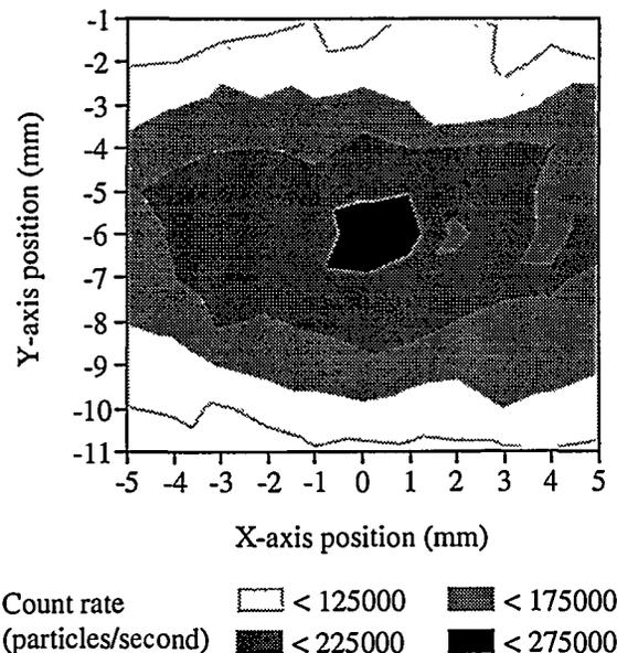
Figure 2. Distribution of particle flow rates within a plume cross-section at 100 mm stand-off. Data collected at "central" conditions (700 A, 18 slpm He, 2.0 slpm carrier gas).
