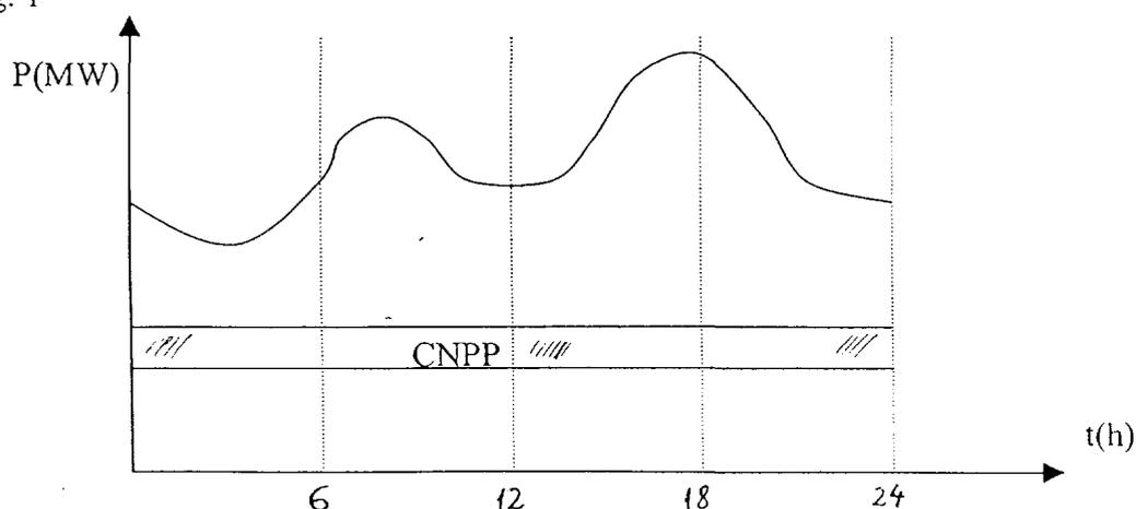
The operation at reduced power is not desirable for C.N.P.P. on the long term due to the fact that the costs per kWh produced are increasing at low power, because the fuel represents only a small contribution to the overall costs while other expenses are rather constant, regardless of power. Investment reimbursement is especially a concern because of the high contribution in the cost.
