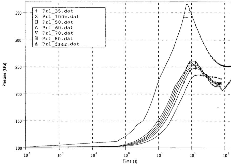
**Figure 6. Containment pressure for spectrum of SLB breaks and USAR MSLB (log scale)**
