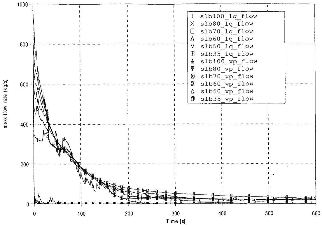
Figure 1. Break Liquid and Vapour Mass Flow Rates
