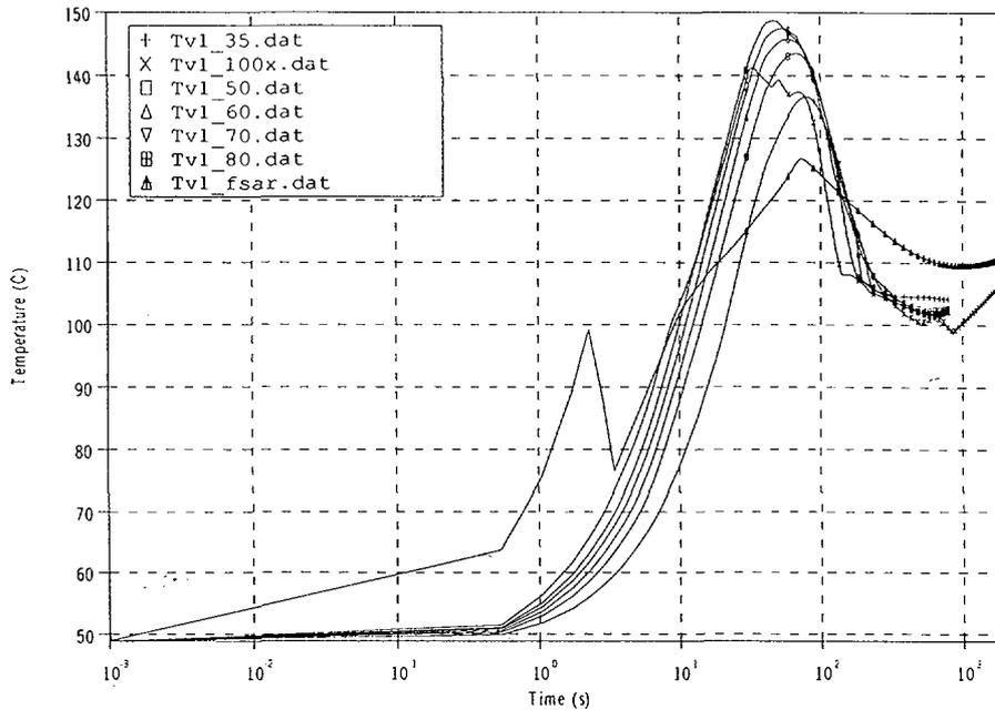
**Figure 8.** Containment temperature for spectrum of SLB breaks and USAR MSLB (log scale)
