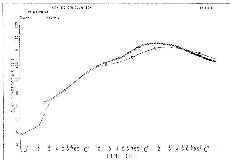
**Figure 5.** *Containment sump temperature used in USAR and calculated by GOTHIC code, double-ended MSLB case*
