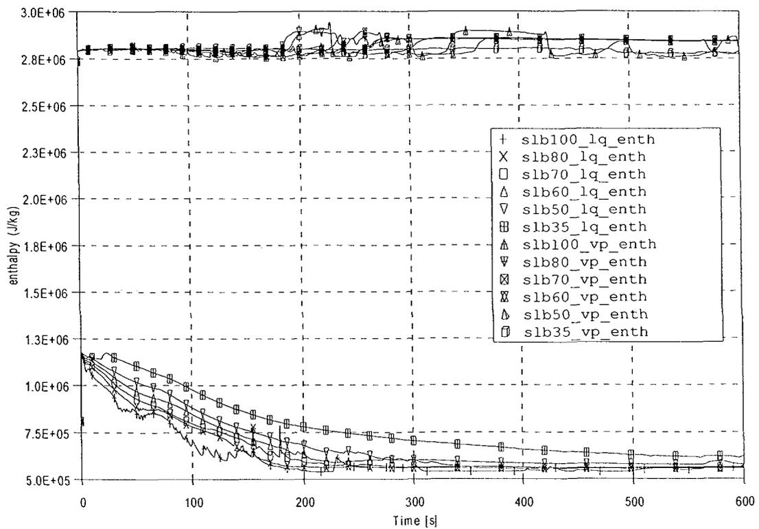
Figure 2. Break Vapour and Liquid Enthalpy
