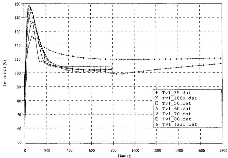
**Figure 9.** Containment temperature for spectrum of SLB breaks and USAR MSLB (lin scale)
