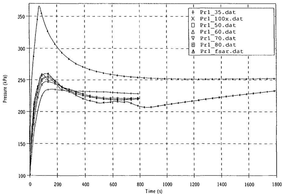
**Figure 7. Containment pressure for spectrum of SLB breaks and USAR MSLB (lin scale)**
