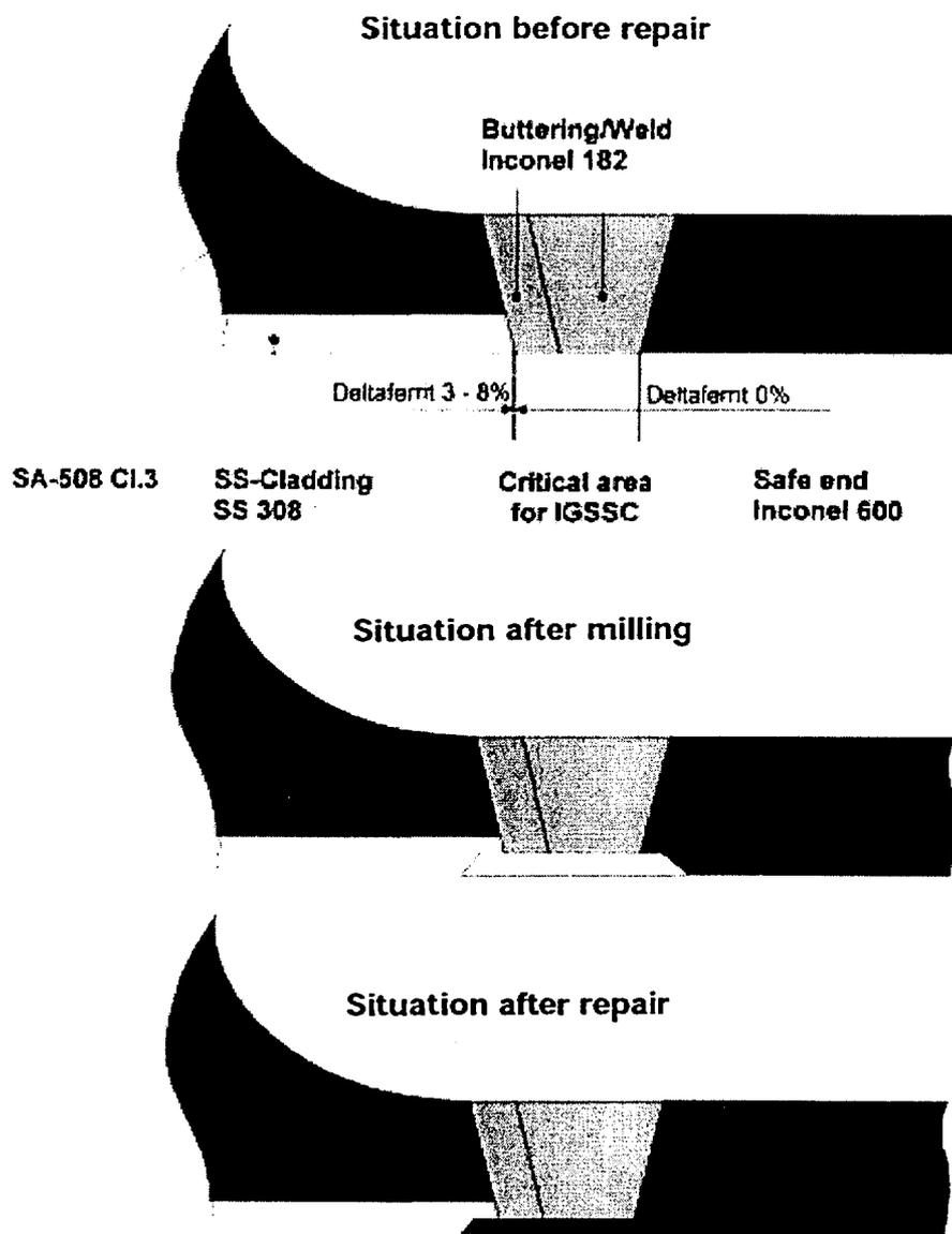
Fig. 4: Nozzle repair from inside
