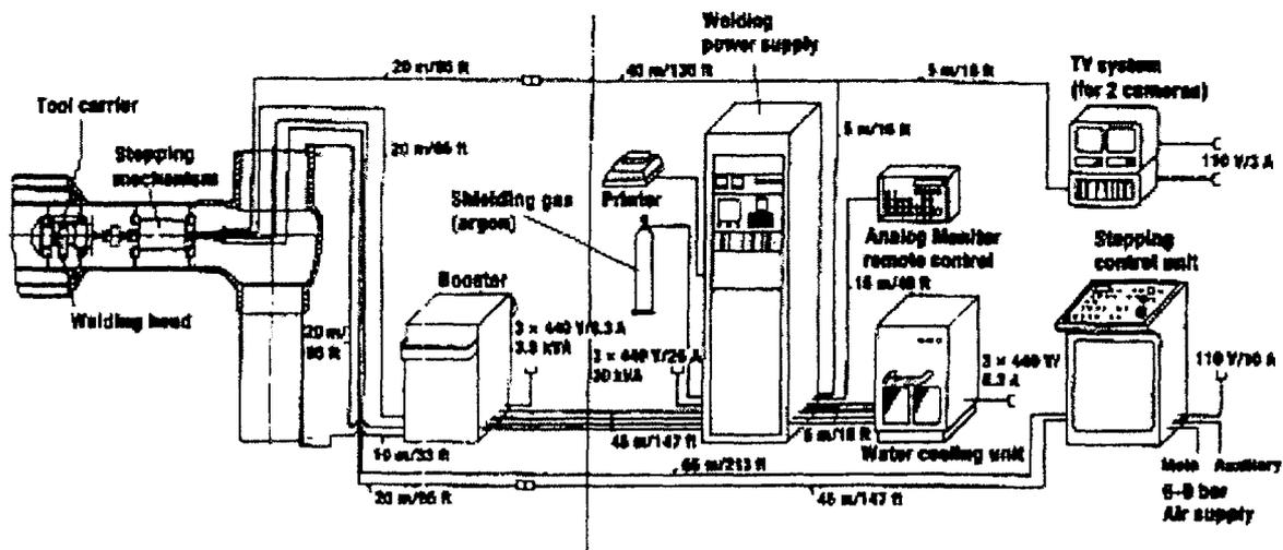
Figure 2: Equipment arrangement for in-pipe welding (sketch)
