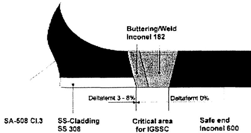
Fig. 1: Detail design of the Nozzle
