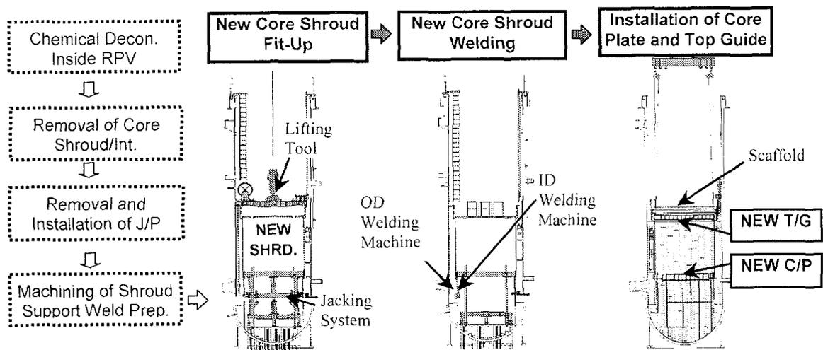
FIG 3. Core shroud replacement sequence.
