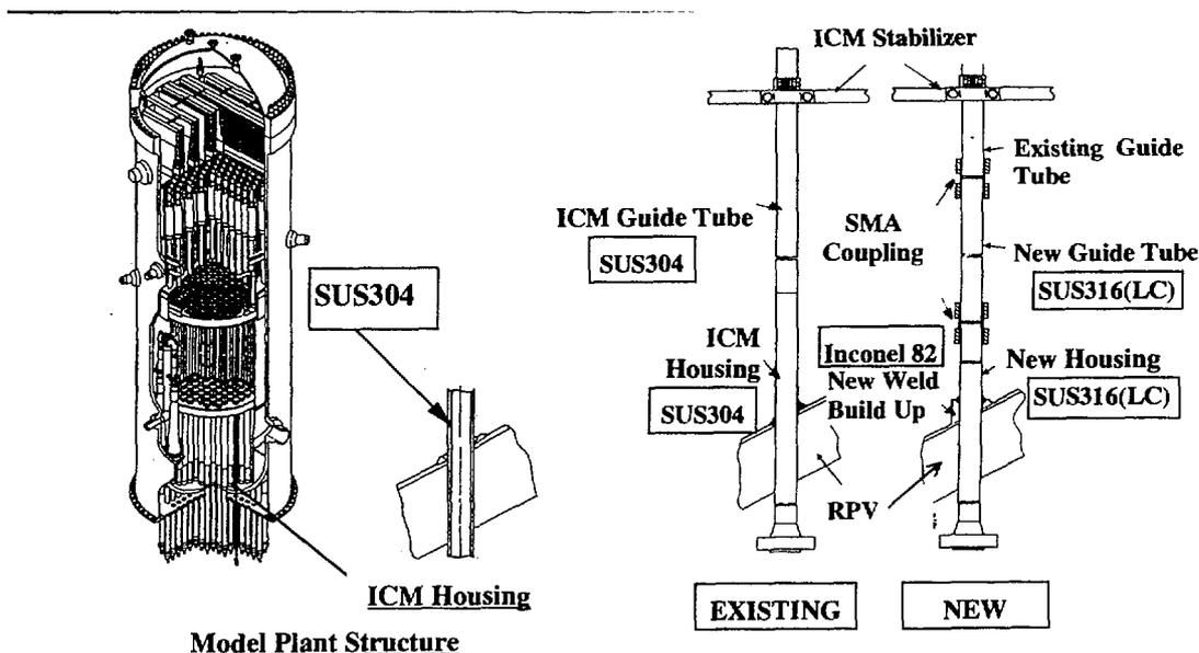
FIG. 6. New ICM housing structure.
