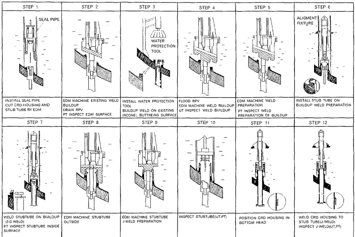
FIG. 11. CRD housing & STUB tube replacement sequence.
