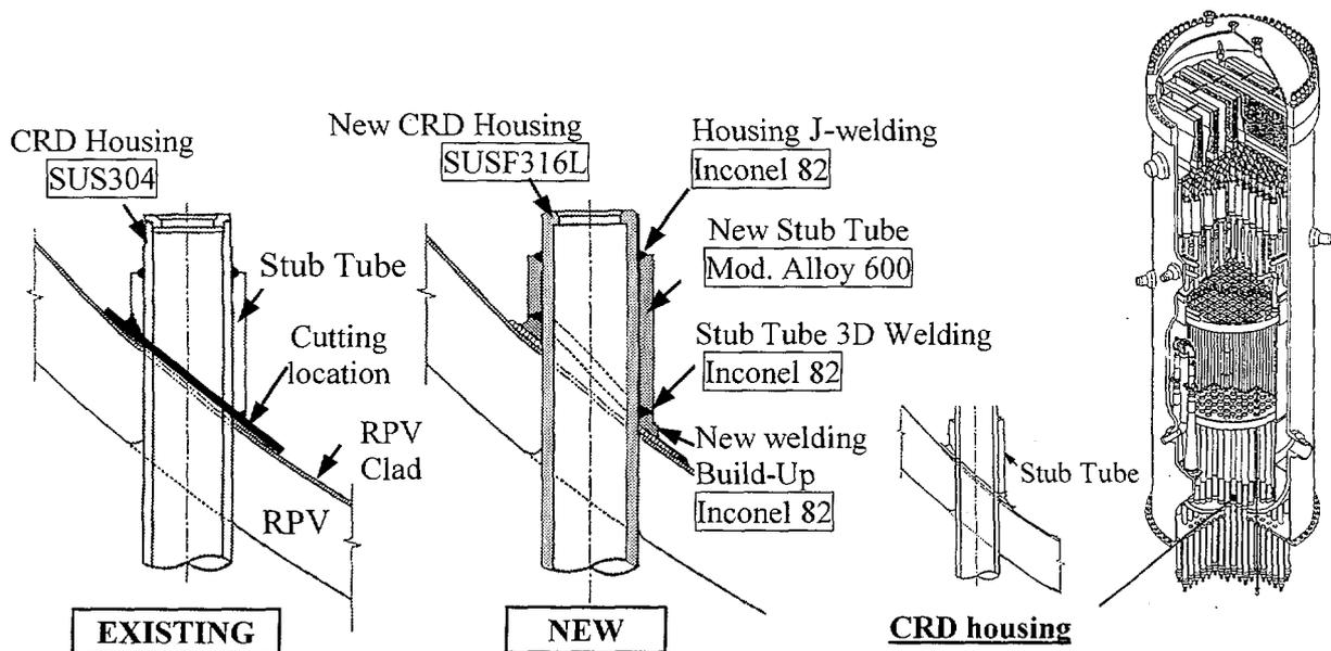
FIG. 10. New CRD housing and stub tube structure.
