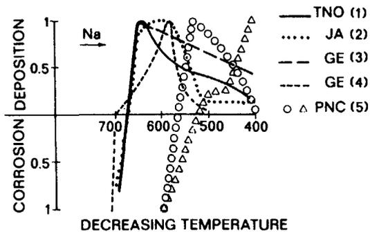
**NORMALIZED DEPOSITION VERS. LOOP TEMPERATURE**
