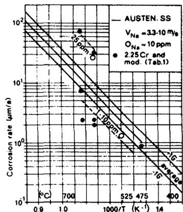
**CORROSION RATE OF FERRITIC AND AUSTENITIC STEELS IN SODIUM**
