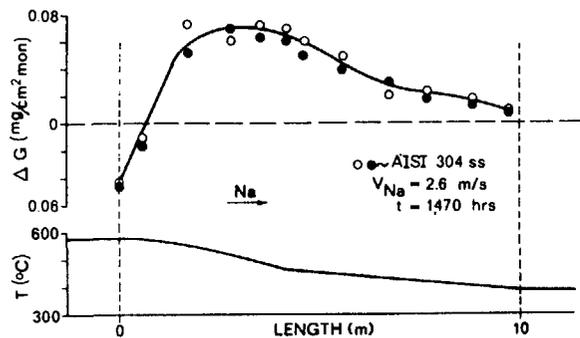
**CORROSION/DEPOSITION IN COOLING SECTION OF SODIUM SYSTEM**
