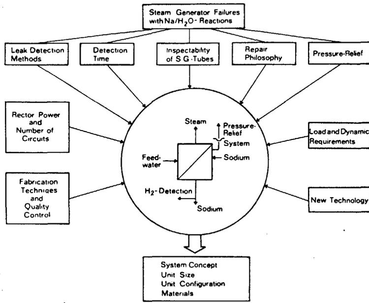
FIG. 2. CRITERIA FOR THE DESIGN OF STEAM GENERATOR SYSTEMS
