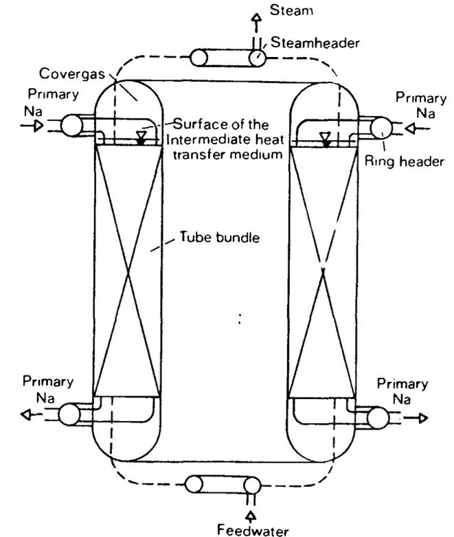
FIG. 5. INTEGRATED "THREE-FLUID STEAM GENERATOR"
