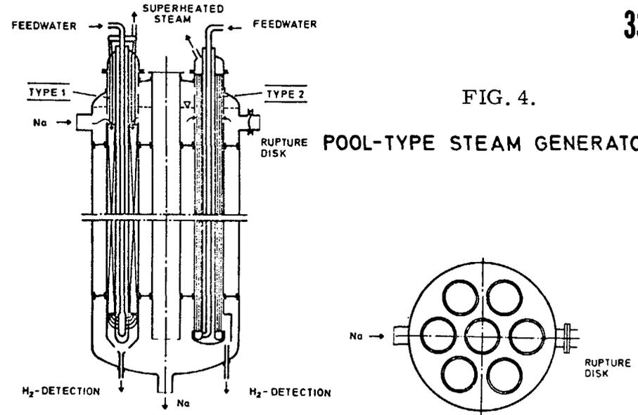
FIG. 4. POOL-TYPE STEAM GENERATOR
