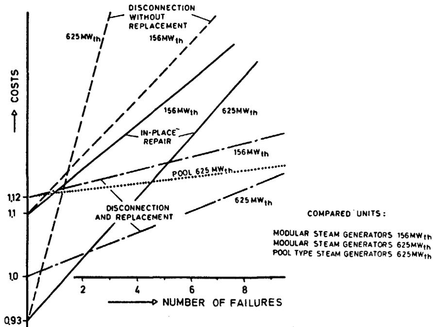
FIG. 3. COSTS OF DIFFERENT REPAIR CONCEPTS
