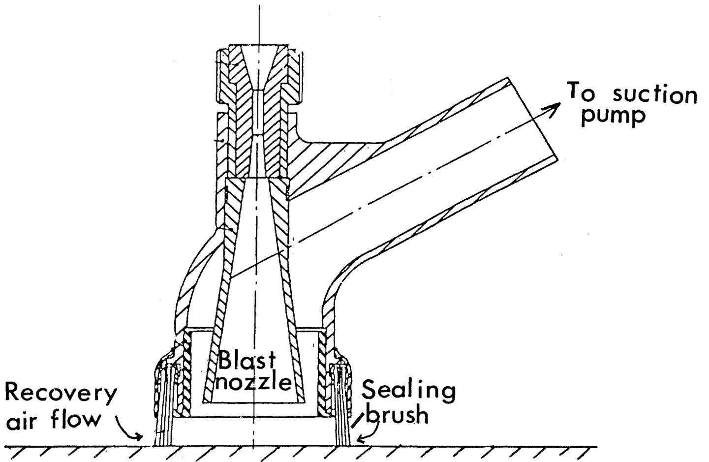
Fig 3 The blast gun with sealing arrangement.
