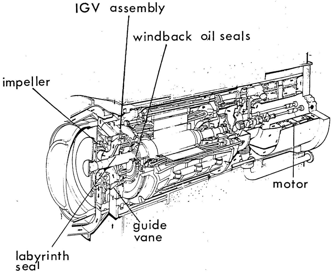
Fig1 General arrangement of the Hinkley Point 'B' gas circulator.
