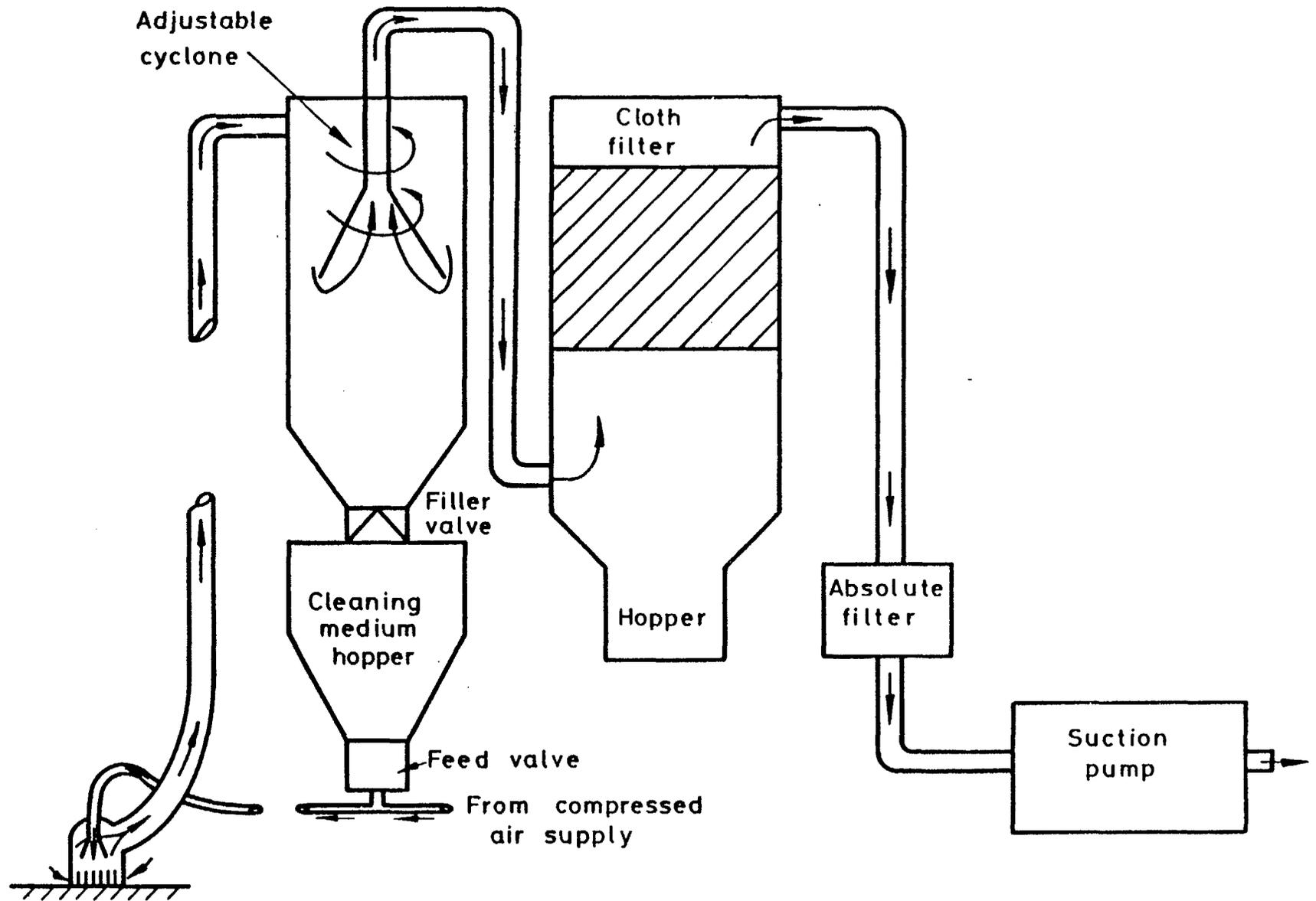
FIG. 2 Schematic Illustration of the Layout of the Vacu-Honer Machine.
