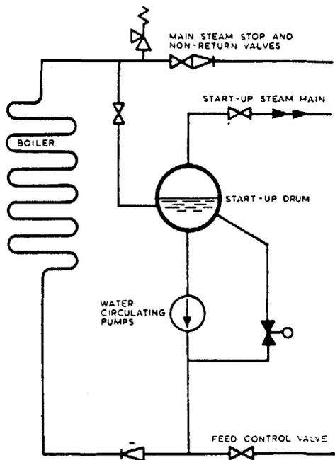
FIG.3. Simplified diagram of boiler start-up system.
