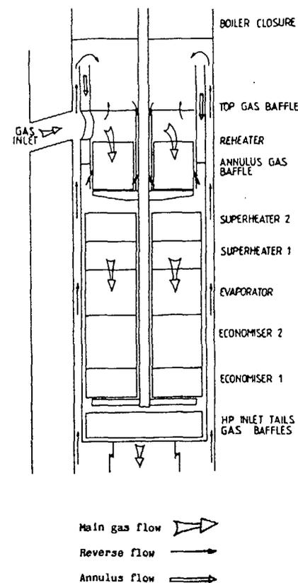
Fig. 1 Pod boiler heating surface arrangement
