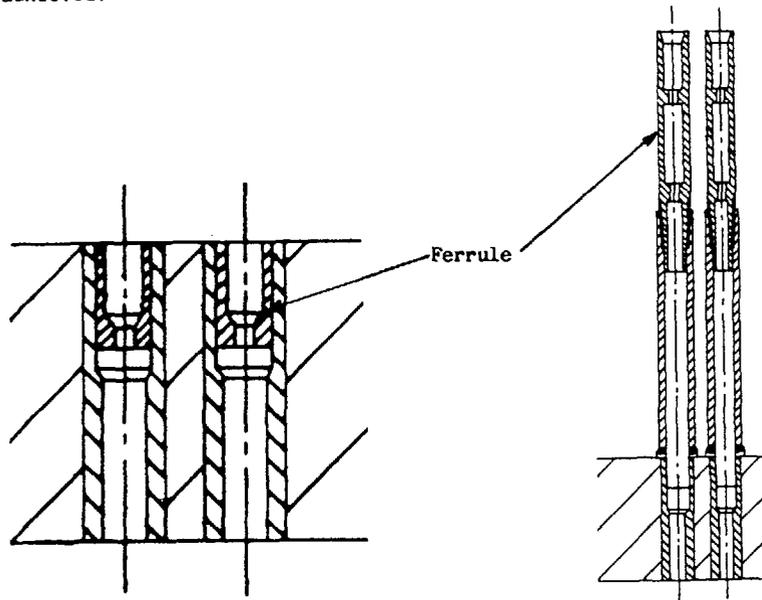
Fig. 2a Original feed flow ferrules Fig. 2b Two stage feed flow ferrules
