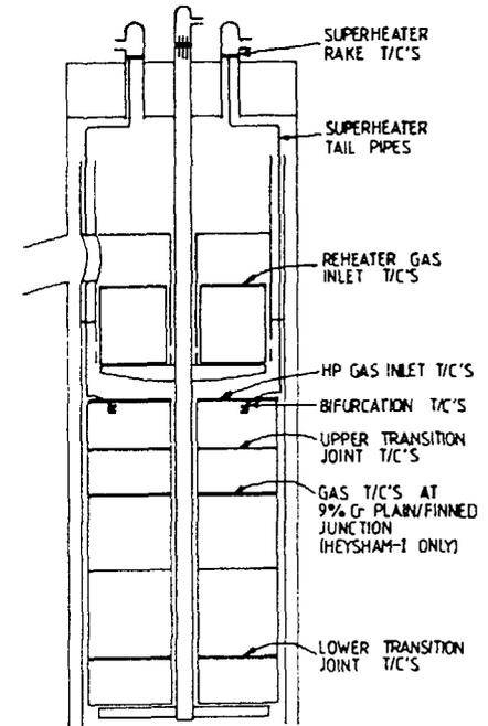
Fig. 3 Thermocouple positions
