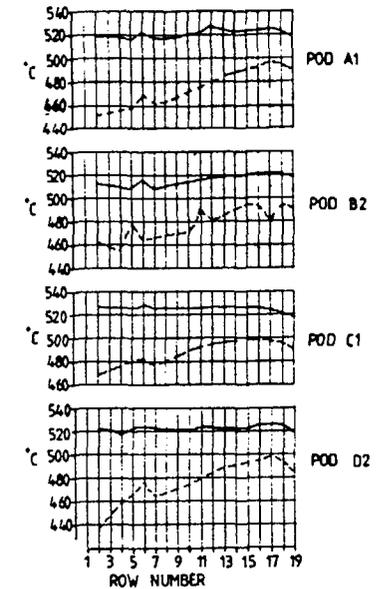
6d Steam Outlet Temperatures before and after refferuling
