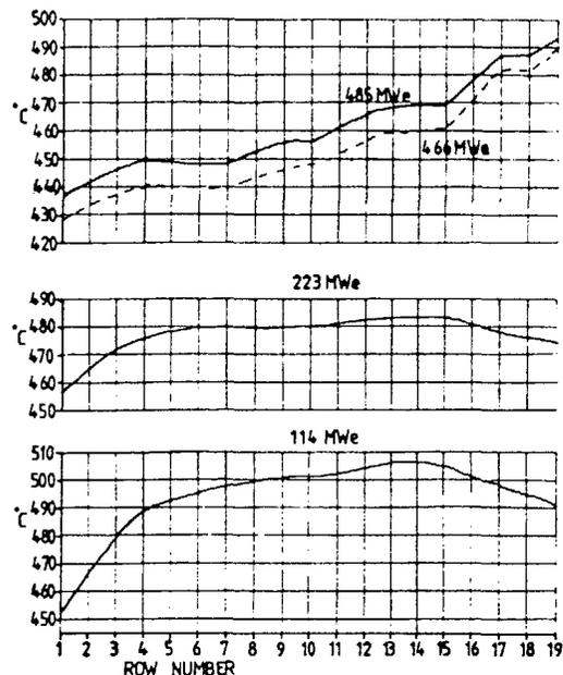
Fig. 7 Heysham R1 UTJ temperature profile at various power levels
