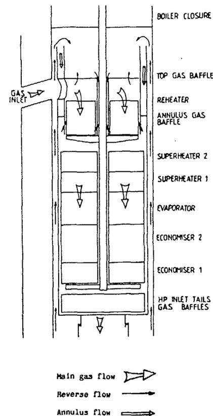
Fig. 1 Pod boiler heating surface arrangement
