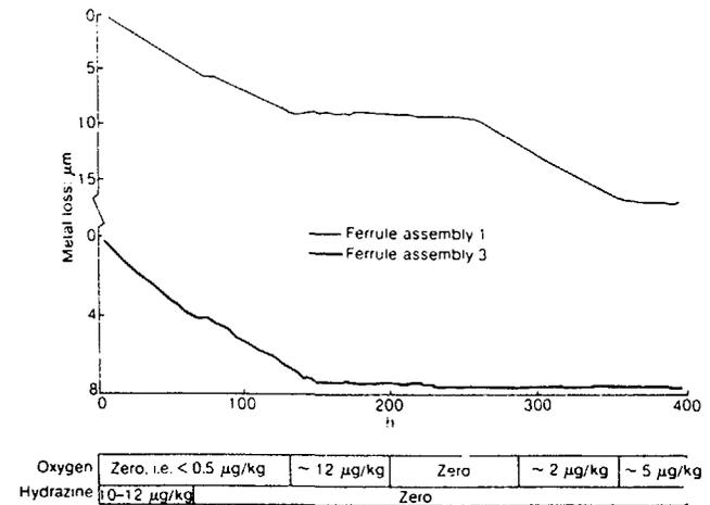
Fig 6 TLA results and the equivalent metal losses on two ferrules with oxygen dosing
