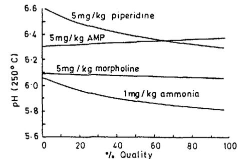
Fig 3 High Temperature pH versus quality for equivalent amine concentrations
