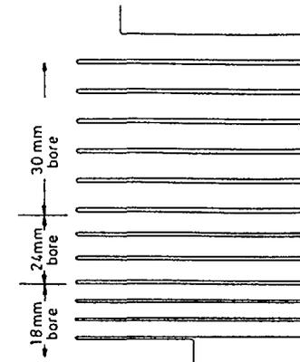
Fig 1 Serpentine Boiler Tube
