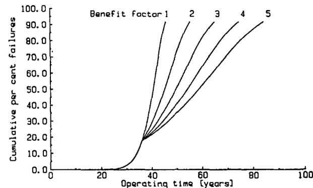
Fig 4 Effect of rate change on failure predictions
