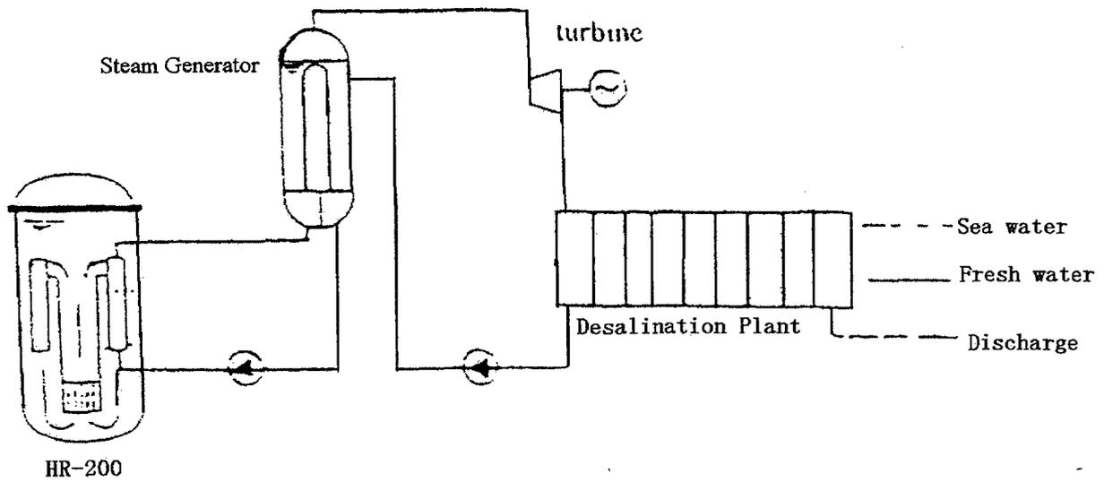
Fig. 3 Back Pressure Cogeneration Plant
