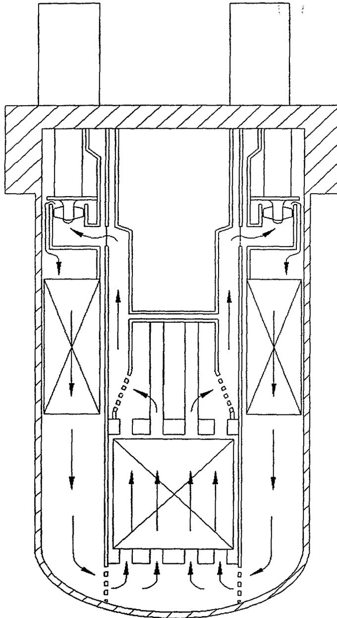
Fig. 2. Primary coolant flow diagram
