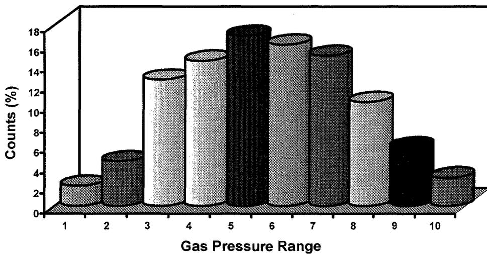
FIG. 16. Histogram of the gas pressure of the free gases in the rod at End of Life (EOL). The columns are between the maximum and minimum calculated values (1.60-2.07 MPa).
