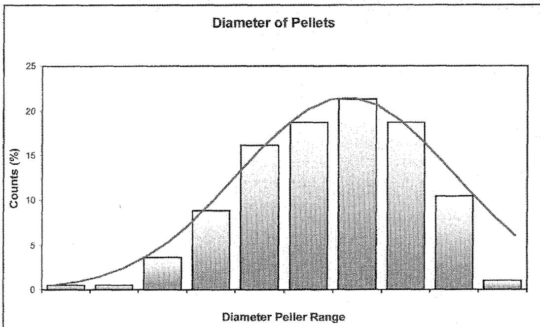
FIG. 8. Histogram of the pellet diameters. The columns are between the maximum and minimum specified values [ $\phi_p = (1.040 \pm 0.001)$  mm]. The curve is the associated Gauss distribution.
