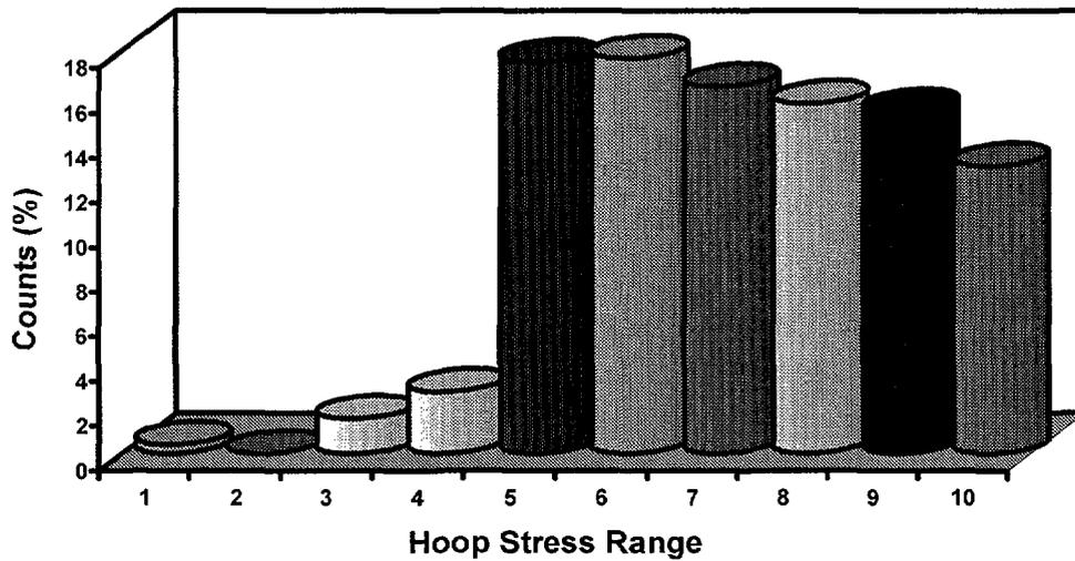
FIG. 14. Histogram of the hoop stress at End of Life (EOL). The columns are between the maximum and minimum calculated values (292-302 MPa).
