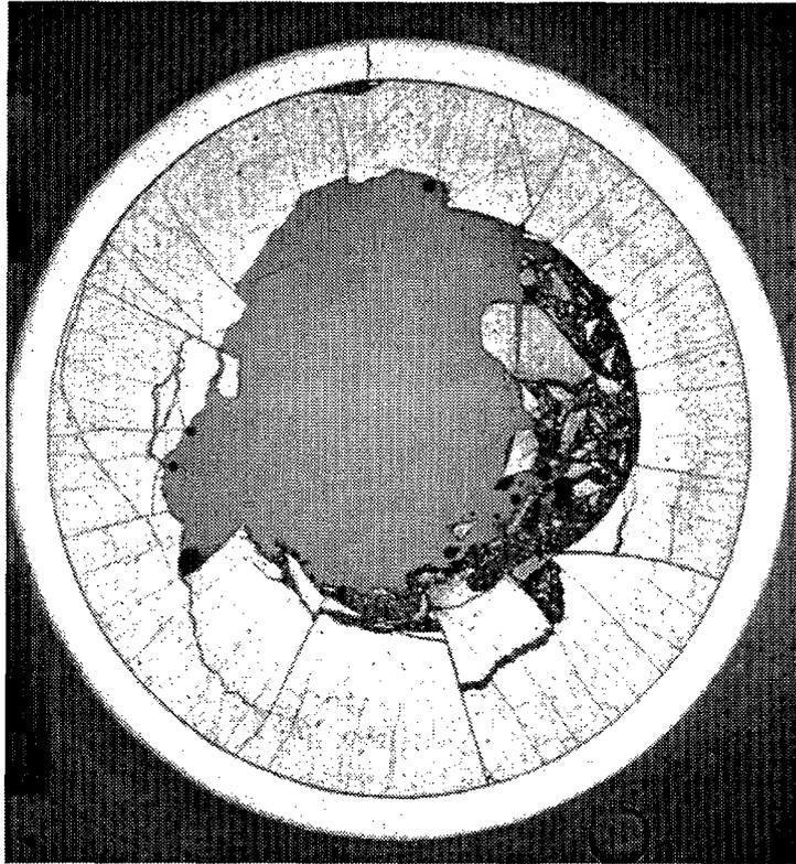
*FIG. 17. Micrograph of a cross section near the defect in rod A.1.3. showing the hole.
