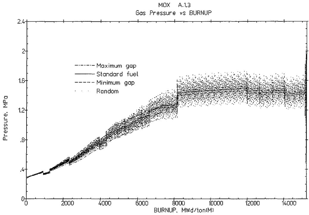
FIG. 15. Gas pressure of the free gases in the fuel rod for the BU15 experiment (A.1.3 rod).
