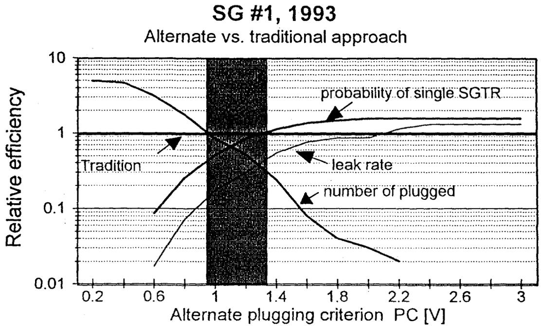
**Figure 1** Comparison of traditional and alternate plugging approach
