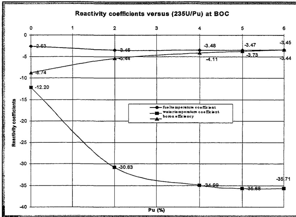
FIG.1A. Reactivity coefficients (at 150 MWd/t) vs. the Pu content
