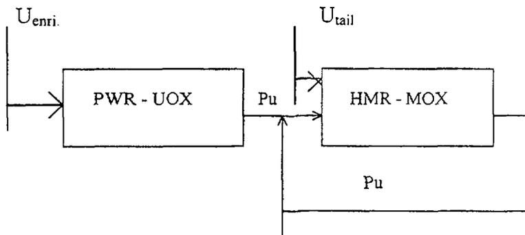
FIG. 3. Pu multirecycling scheme with the HMR
