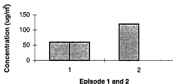
Figure 3: Comparison of two episodes with different duration and peak height, but with similar total integrated exposure ( 120 \mu\text{g}/\text{m}^3 hours).
