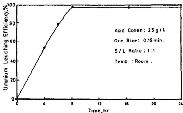
Figure (2) : Effect of Time upon Uranium Leaching Efficiency of Wadi Belih Ore Material
