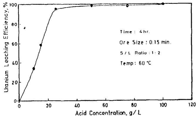
**Figure (1) : Effect of Sulphuric Acid Concn. on Uranium Leaching Efficiency of Wadi Belih Ore Material**
