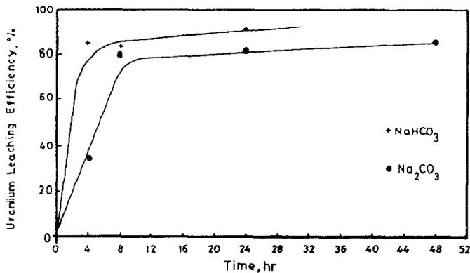
**Figure (6) :** Effect of Alkaline Leaching Temp. on Uranium Leaching Efficiency of Wadi Belih Ore Material
