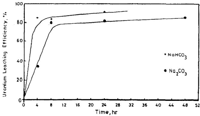
**Figure (5) :** Effect of Alkaline Leaching Time on Uranium Leaching Efficiency of Wadi Belih Ore Material
