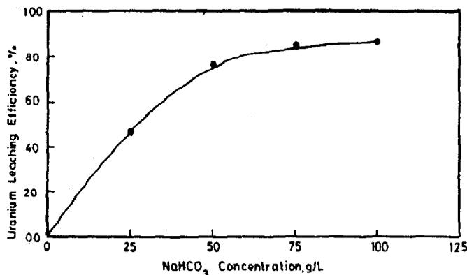
**Figure (4) :** Effect of Carbonat Conc. on Uranium Leaching Efficiency of Wadi Belih Ore Material
