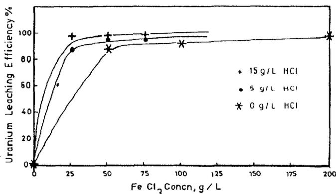
**Figure (8) :** Effect of Ferric Chloride Concn, on Uranium Leaching Efficiency of Wadi Belih Ore Material
