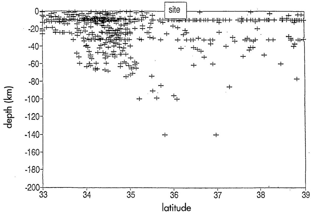
Figure 4. Depths of Earthquakes from 1900-1988. Section N-S.
