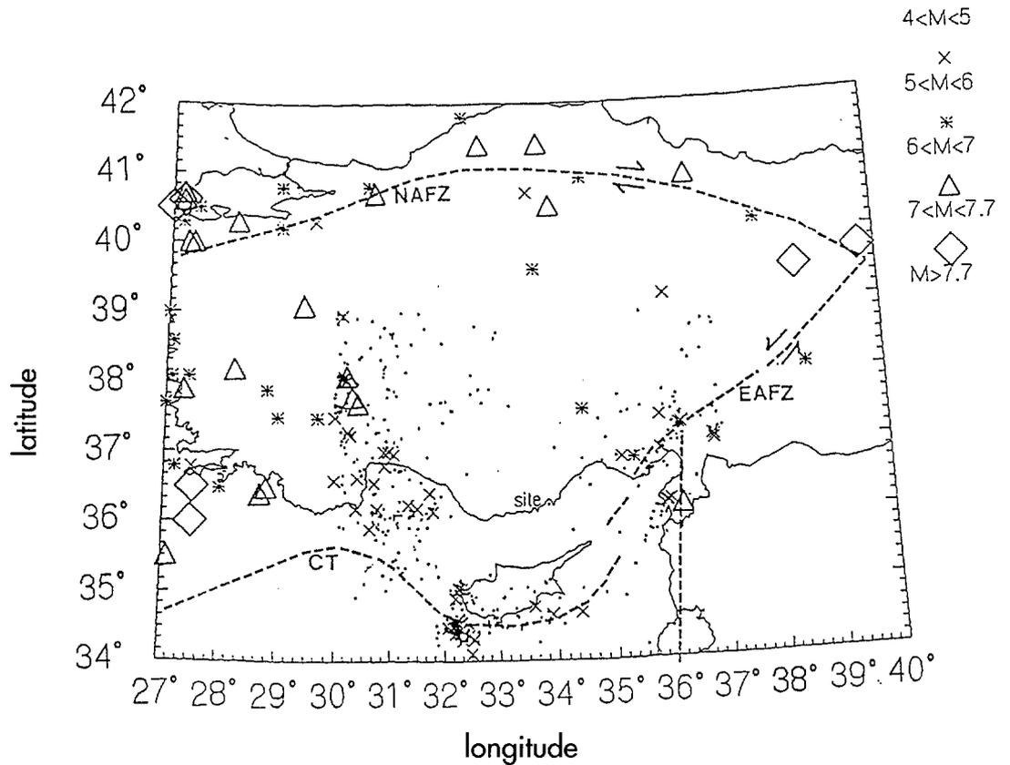
Figure 3. Significant Earthquakes in the Mapped Region, Plus All Events of  $M > 4$  since 1963. Approximate locations of plate boundaries are shown.
