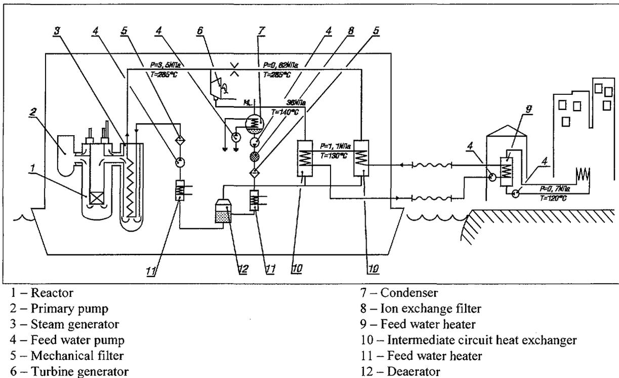
FIG. 2. Schematic flow diagram of NCGP with the shore heat supply system.
