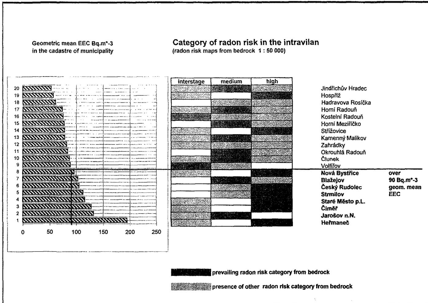
Fig. 7 - The comparison of mean indoor radon (EEC) with radon risk from bedrock in South-Bohemian municipalities situated on the crystalline and granitic bedrock
