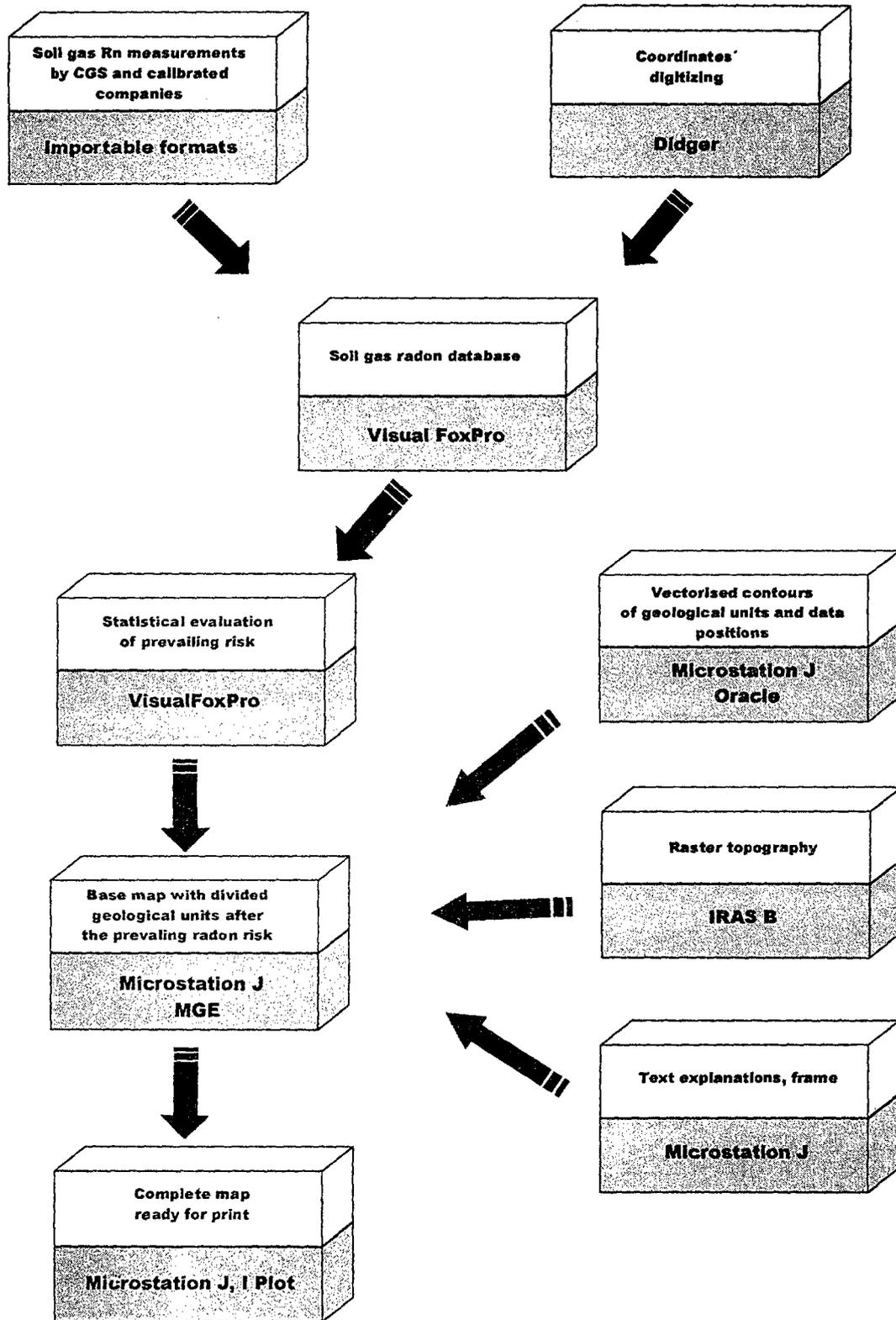
Fig. 3 - The flowchart diagram of creation of radon risk maps on a scale 1 : 50 000
