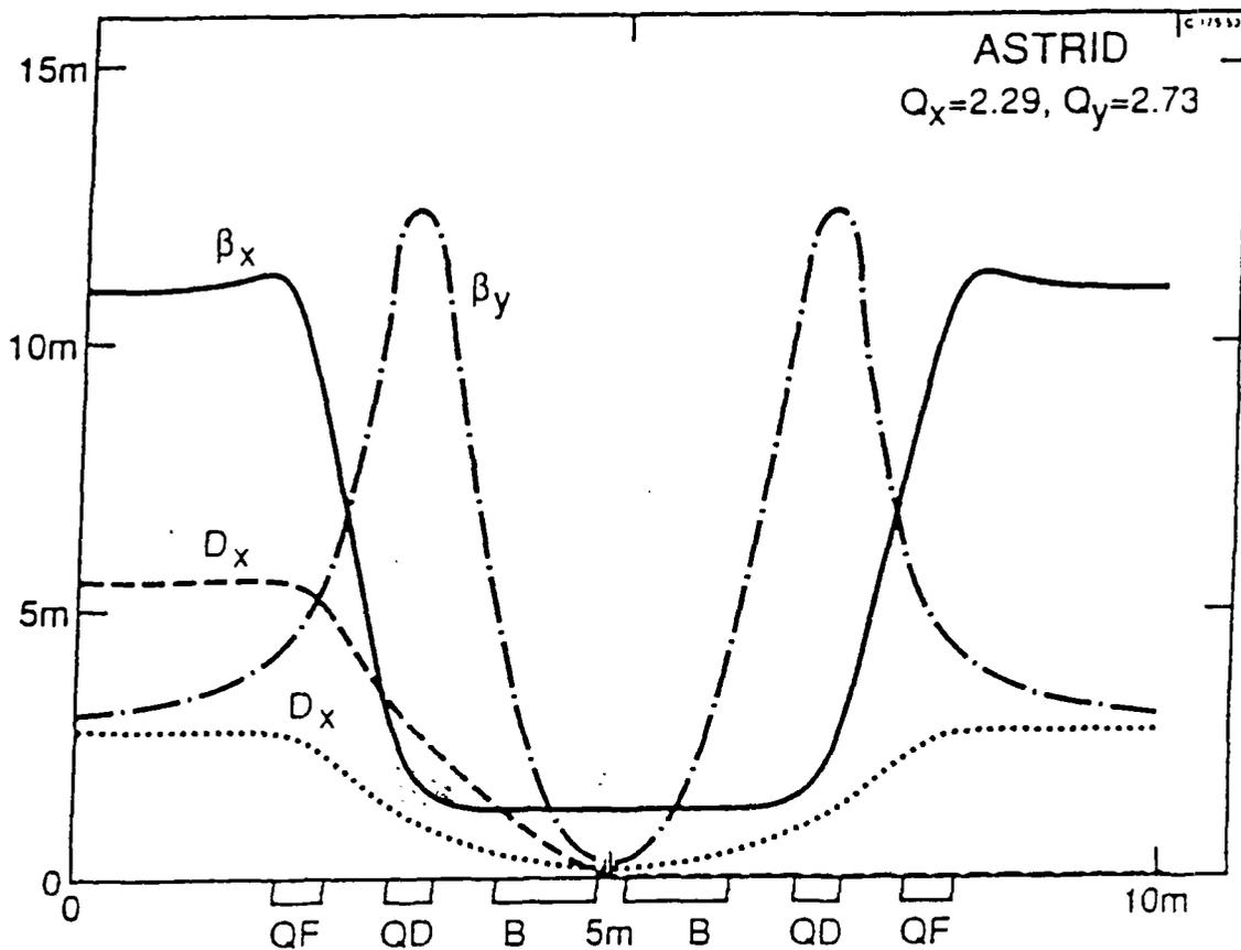
FIGURE 2. The Lattice Functions in ASTRID
