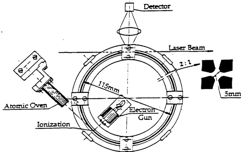
FIGURE 6. The Ion Trap. (The Quadrupole Storage Ring).
