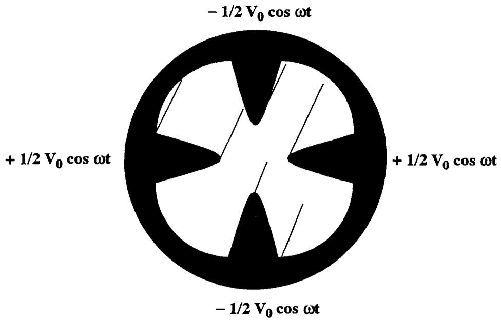
**FIGURE 4.** Cross-section of a RFQ
