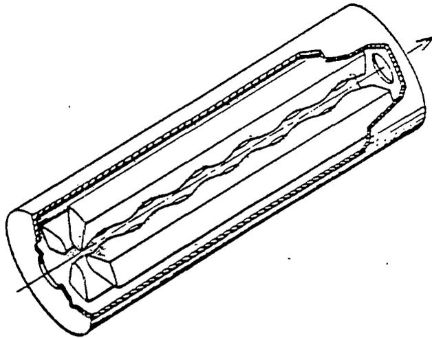
FIGURE 3. Four-Vane RFQ (Linear) Corrugated Structure
