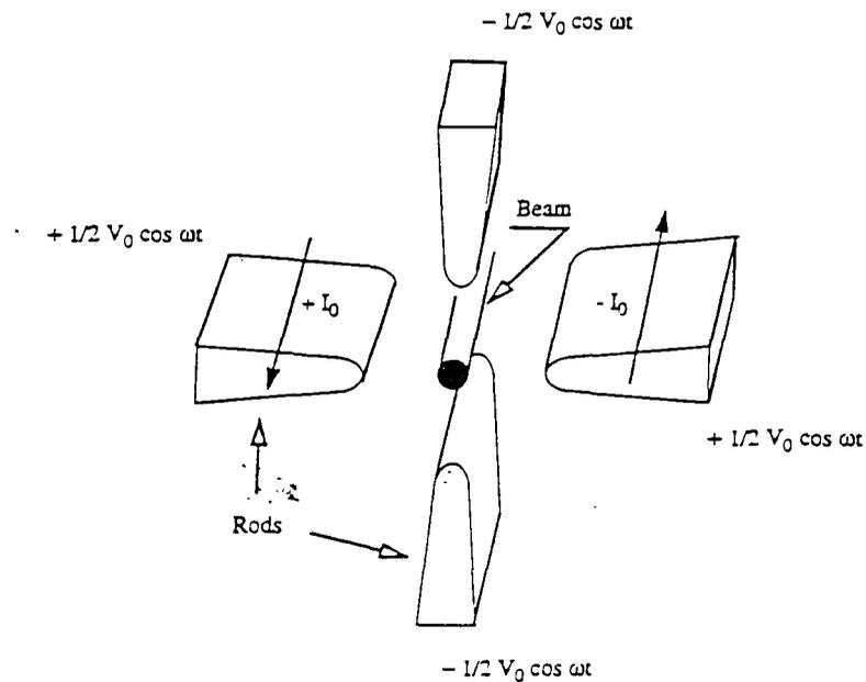
FIGURE 9. Cross-section view of the CRFQ. A transverse rf field is excited between the electrodes. The rf excitation is as shown. DC current  $I_0$  flows along the outer electrodes generating a magnetic field to bend the beam circulating in the region inside.
