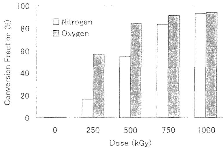
Fig.1 Pulverization of Irradiated Silk Fiber(degummed)
