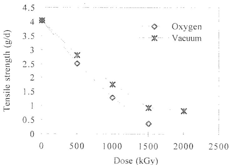
Fig.1 Tensile strength of irradiated silk fibroin fibers
