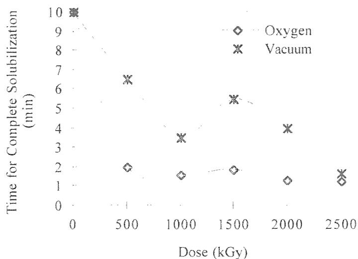
Fig.2 Radiation Effect on dissolution of silk fibroin fibers in the calcium chloride solution( $\text{CaCl}_2/\text{C}_2\text{H}_5\text{OH}/\text{H}_2\text{O}=1:2:8$  in mole ratio).
