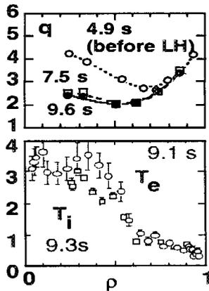
Figure 4: Spatial profiles of  $q$  before and during LHCD (top box), and  $T_e$  and  $T_i$  profiles at the later phase of LHCD.
