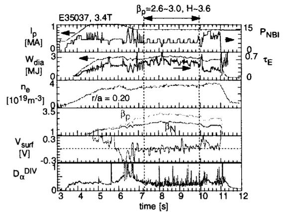
Figure 5: Wave forms of a high bootstrap current fraction RS discharge;  $I_p$ ,  $P_{NB}$ ,  $W_{dia}$ ,  $\tau_E$ ,  $n_e$  at  $r/a = 0.2$ ,  $\beta_N$ ,  $\beta_p$ ,  $V_{surf}$  and  $D_{\alpha}$ .
