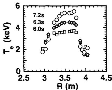
Figure 8: Changes of the  $T_e$  profile by fundamental O-mode central ECH in a RS plasma;  $I_p = 1.2$  MA,  $P_{NB} = 5$  MW,  $R_{axi} = 3.41$  m,  $a_p = 0.83$  m,  $n_{e0} \sim 3 \times 10^{19} \text{m}^{-3}$  and  $T_{i0} \sim 7$  keV at 6.0 s. ECRF was injected from 6.0 s.
