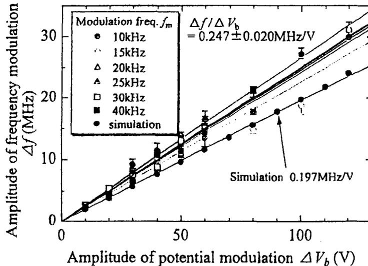
Fig. 5 Experimental and simulation results for frequency modulation amplitude  $\Delta f$  versus the amplitude of body potential modulation  $\Delta V_b$  for  $f_m=10, 15, 20, 25, 30$  and  $40$  kHz. Observed frequency modulation efficiency  $\Delta f/\Delta V_b=0.247$  MHz/V. Output power  $P=20$  W.
