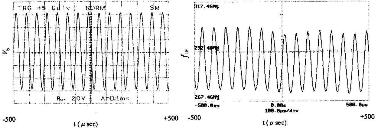
Fig. 4 Typical experimental results of frequency modulation. The traces show the modulation of  $V_b$  (in the left hand side) and the modulation of the output frequency which is demonstrated by the modulation of  $f_{IF}$  (in the right hand side)  $f_m=15$  kHz,  $\Delta V_b=120$  V and  $\Delta f=31.1$  MHz.
