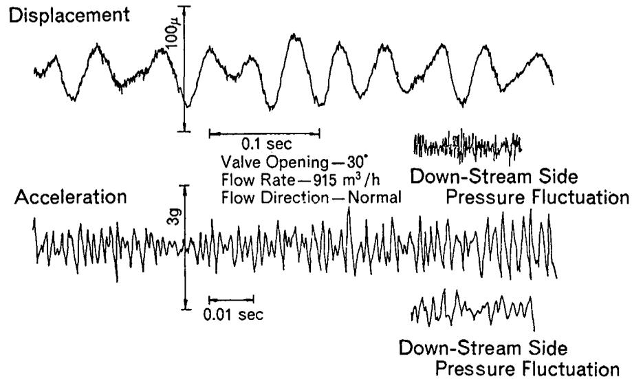
Fig. 21 Vibration Waveform Recorded on an Electro-Magnetic Oscillograph
