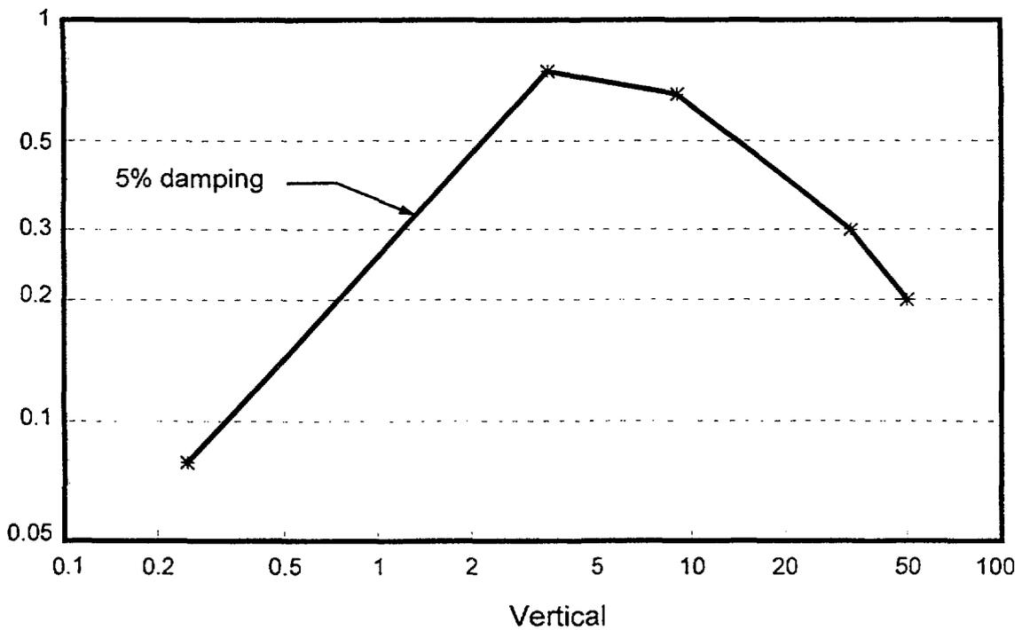
Figure 2: Interim Review Level Earthquake for Bohunice
