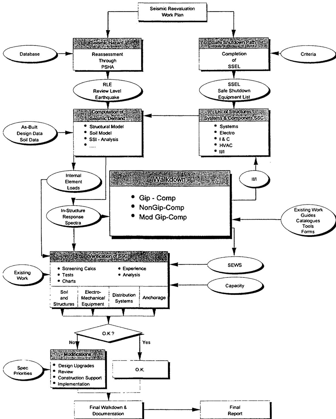
Figure 1: Flowchart for Seismic Verification of SSCs
