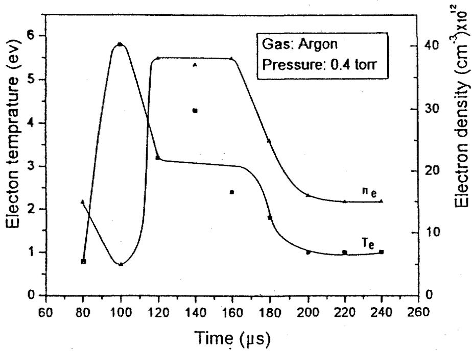
Fig ( 4 ) : The variation of the electron temperature And density of the ejected plasma with time .
