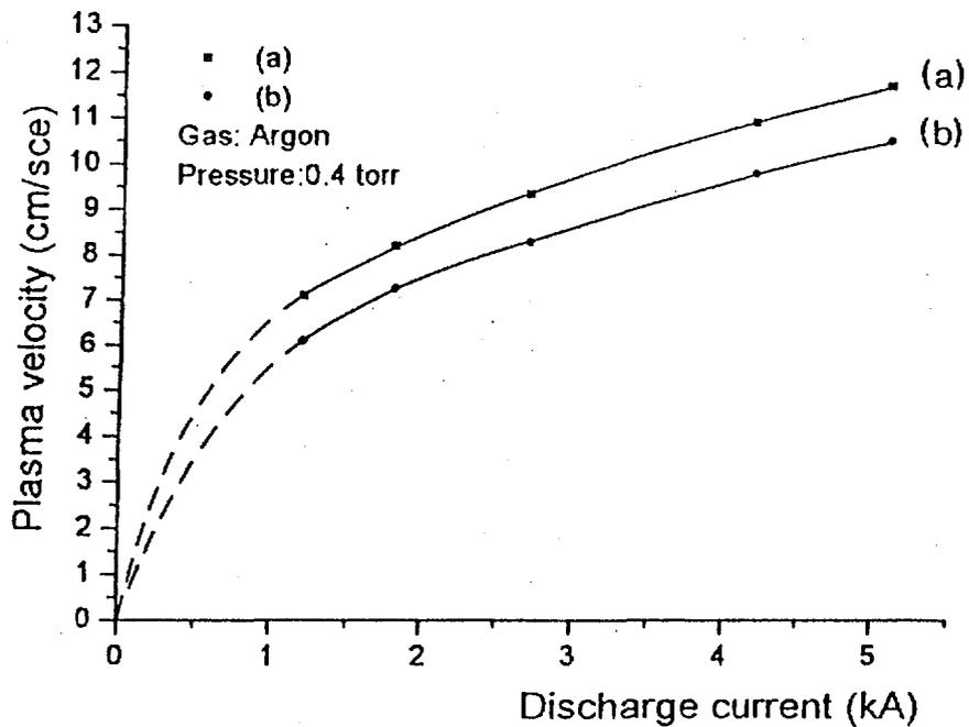
Fig ( 5 ) : The variation of ejected plasma sheath velocity Versus discharge current .
