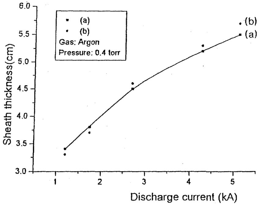
**Fig (6 ) The variation of plasma sheathg thickness versus discharge current, with and without negative glow region.**
