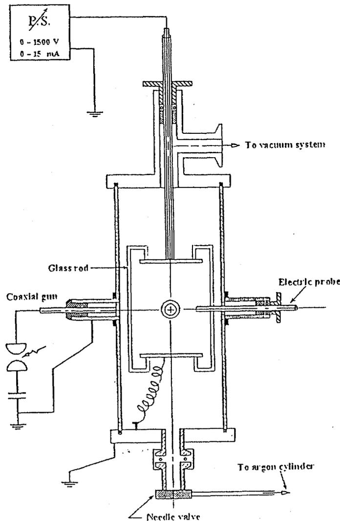
Fig (1) : Schematic diagram of the experimental system
