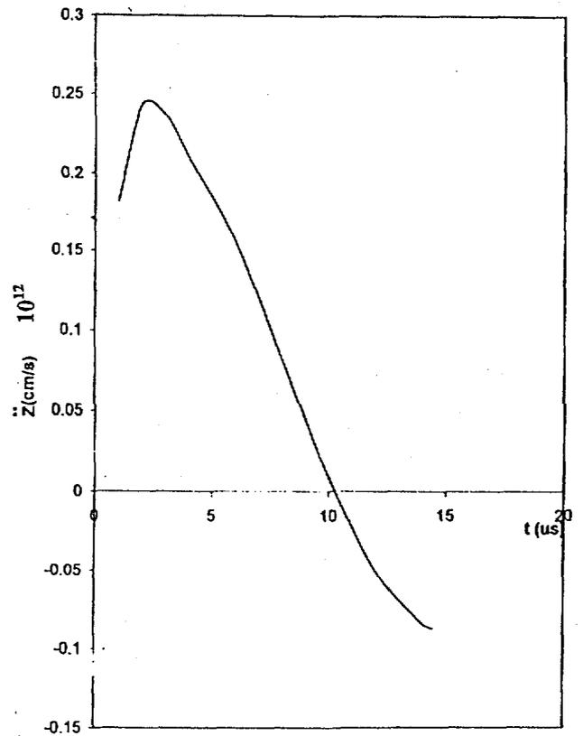
Fig(2c) Axial plasma current sheath acceleration versus time
