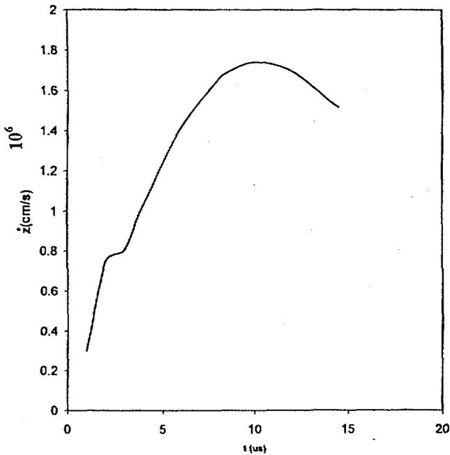
Fig (2b) Axial plasma current sheath velocity versus time
