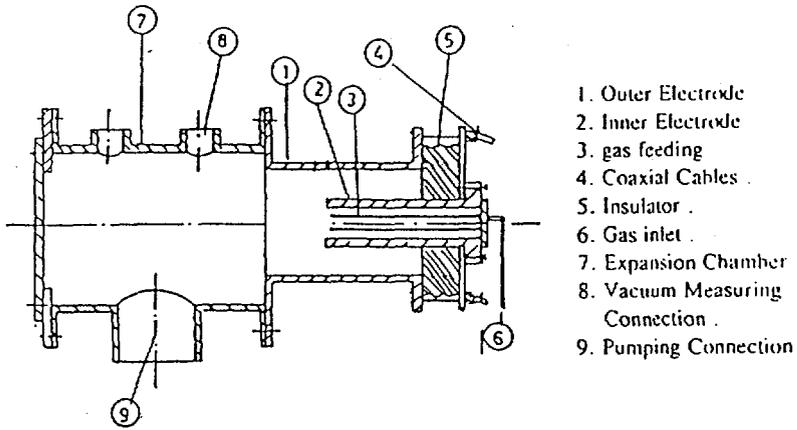
Fig (1) Cross section of coaxial electrodes.
