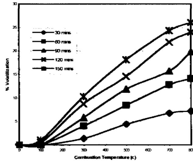
**FIGURE 2 % Volatilization Ra-226 VS Combustion Temperature (°C)**
