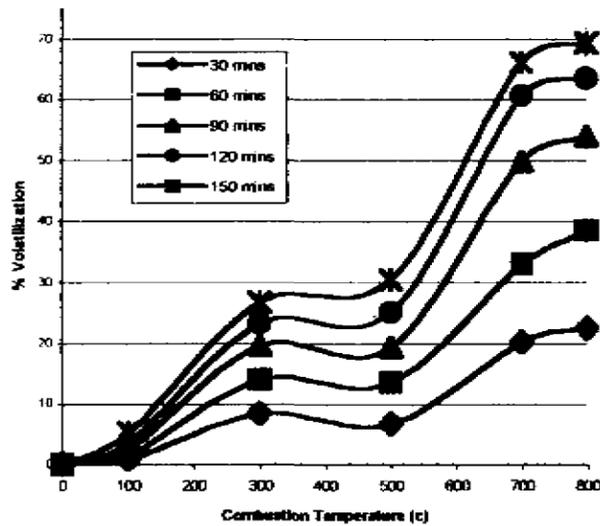
**FIGURE 1 % Volatilization U-238 VS Combustion Temperature (°C)**
