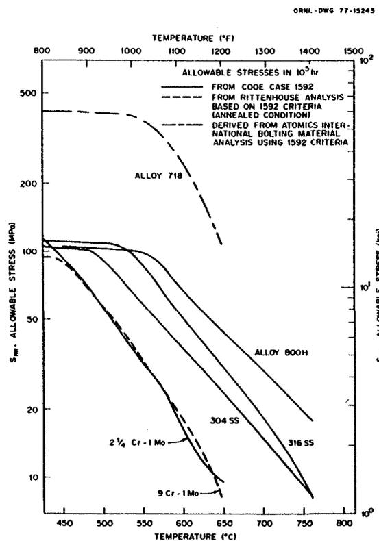
Fig. 1. Comparison of ASME Allowable Stress Levels For Various Alloys in (Solid Lines) or Under Consideration for ASME Code Case 1592.
