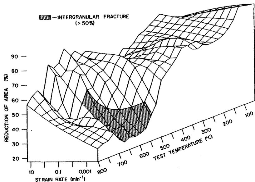
Fig. 6. Creep-Rupture Ductility, Measured as Reduction of Area, as a Function of Temperature and Strain Rate for Type 304 Stainless Steel.
