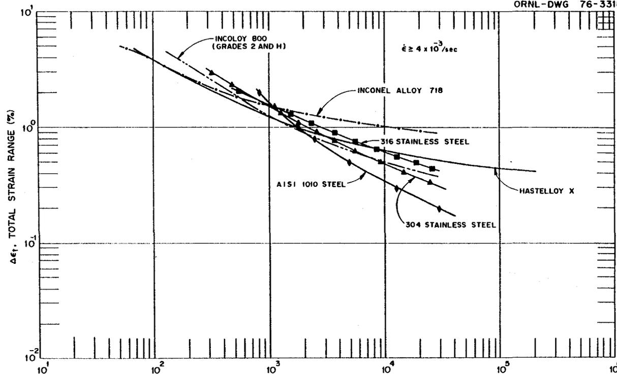
Fig. 2. Comparison of the Fatigue Behavior of Several Materials at 649°C. Lines represent best-fit values of actual data. Advantage of use of alloy 718 for high-cycle fatigue resistance are apparent.
