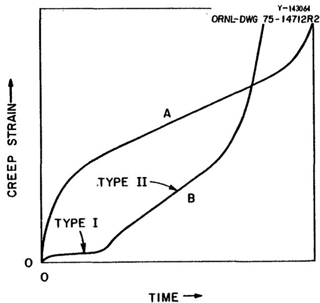
Fig. 4. Schematic Diagram Comparing Classical (A) and Nonclassical (B) Creep Curves.
