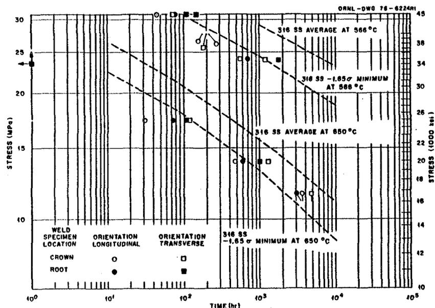
Fig. 8. Comparison of Creep-Rupture Properties of Type 16-8-2 Stainless Steel Submerged-Arc-Weld Specimens With Type 316 Stainless Steel Base Metal.
