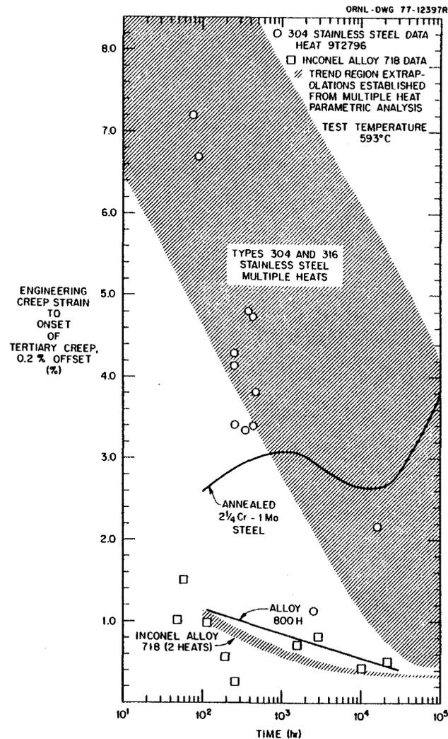
Fig. 5. Comparisons of Tertiary Creep Strain Trends for Several Materials at 593°C. Trend regions are only approximate.
