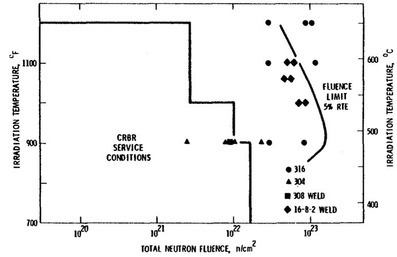
Fig. 10. Irradiation Conditions for Current Experiments on Stress Rupture of Austenitic Stainless Steel.
