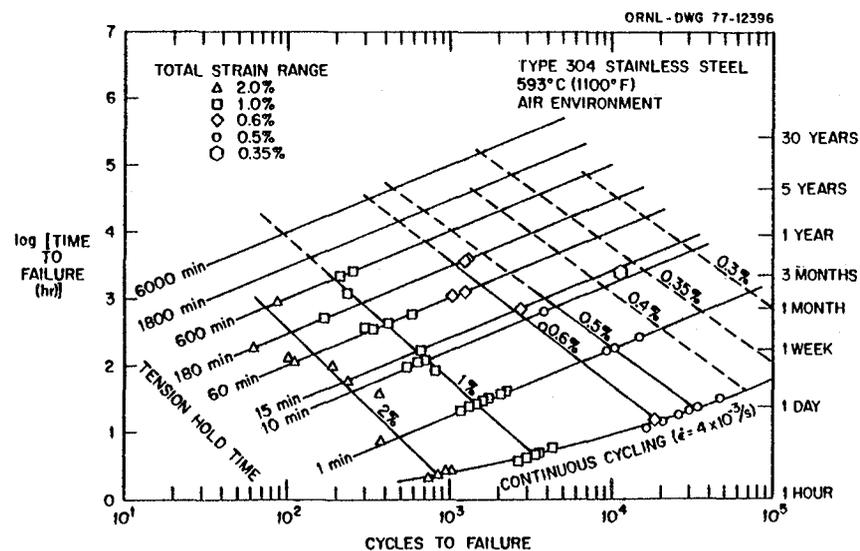
Fig. 7. Time to Failure Versus Cycles to Failure Diagram Showing That Only Data From Essentially Short-Term Tests Are Available for Characterizing Time-Dependent Fatigue of This Material.
