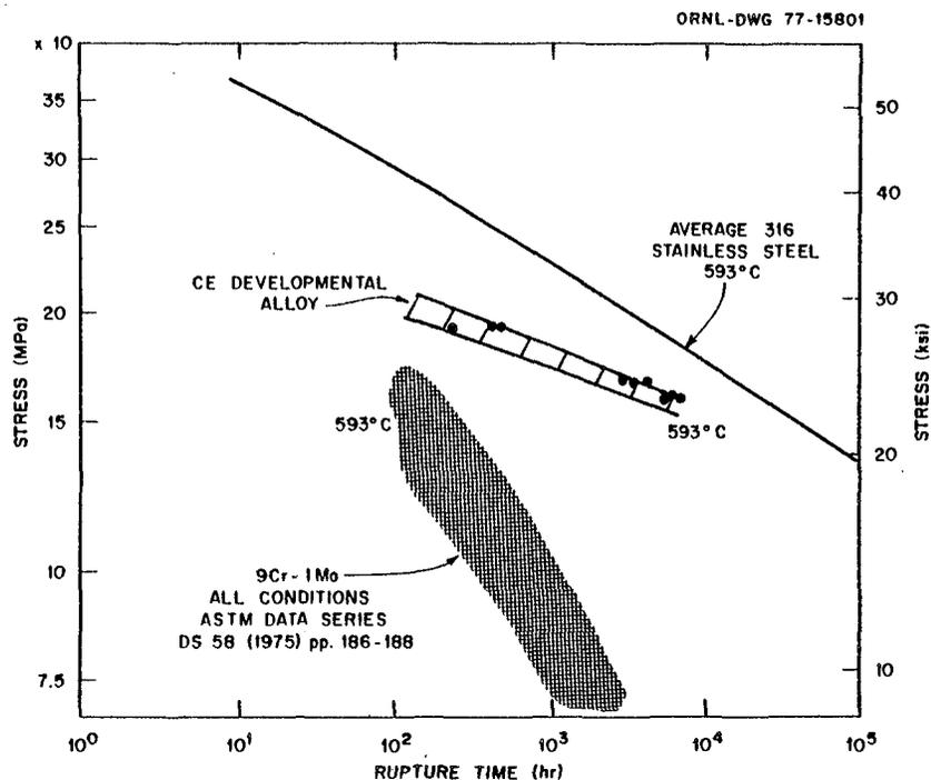
Fig. 3. Comparison of Stress-Rupture Behavior of Combustion Engineering Developmental 9 Cr-1 Mo (Low C, -W, -Nb, -B, -N) steel in the Normalized-and-Tempered Condition With Commercial 9 Cr-1 Mo and Type 316 Stainless Steel.
