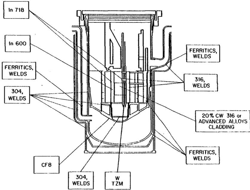
Fig. 9. Schematic Drawing Showing Reactor Structural Materials Undergoing Irradiation Exposure for Mechanical Properties Tests.
