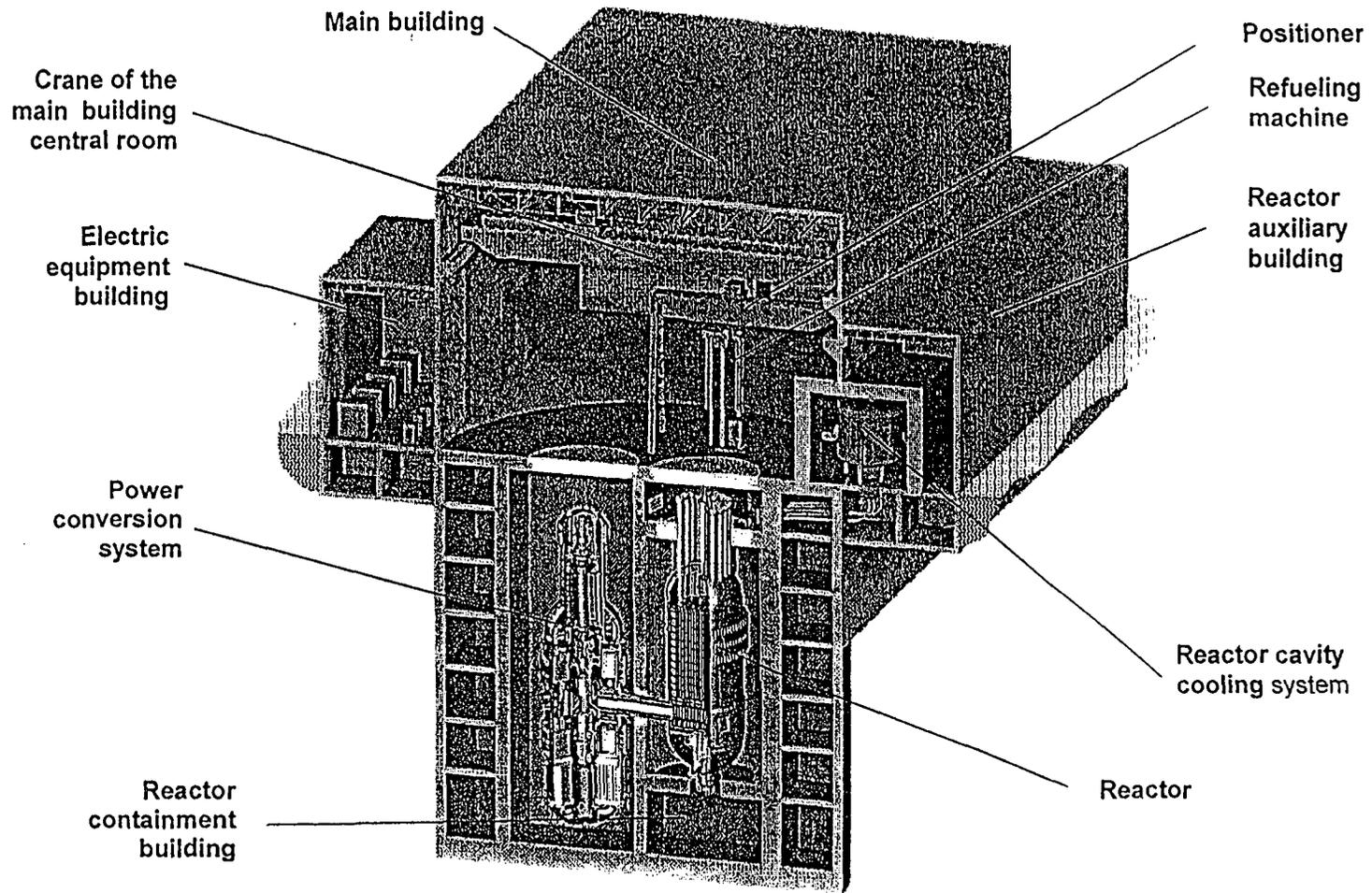
FIG. 1. GT-MHR reactor module arrangement in reactor building.
