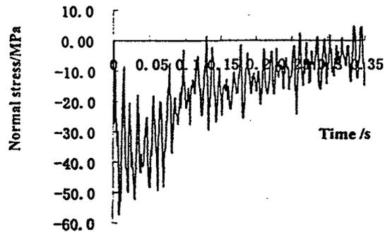
Figure 7 Normal stress in the axial section
