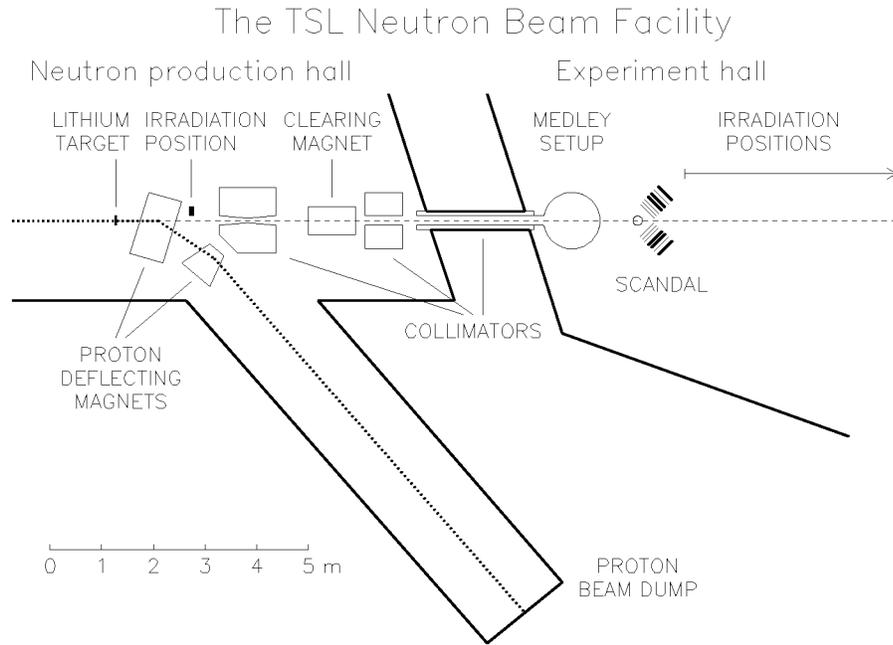
Figure 1: Overview of the Uppsala neutron beam facility.
