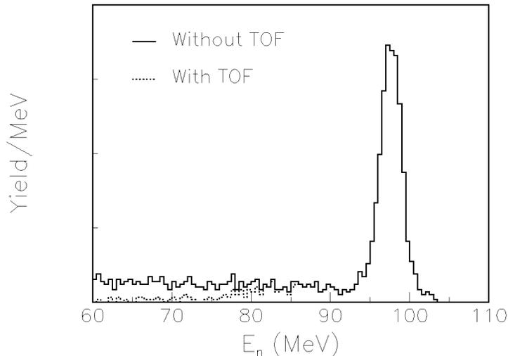
Figure 3: Reconstructed energy spectra of incoming neutrons, using a proton spectrum in the angular range  $0 - 5^\circ$  measured with the LISA magnetic spectrometer. The solid line shows the spectrum without time-of-flight conditions, and the dashed spectrum is obtained with such a cut.
