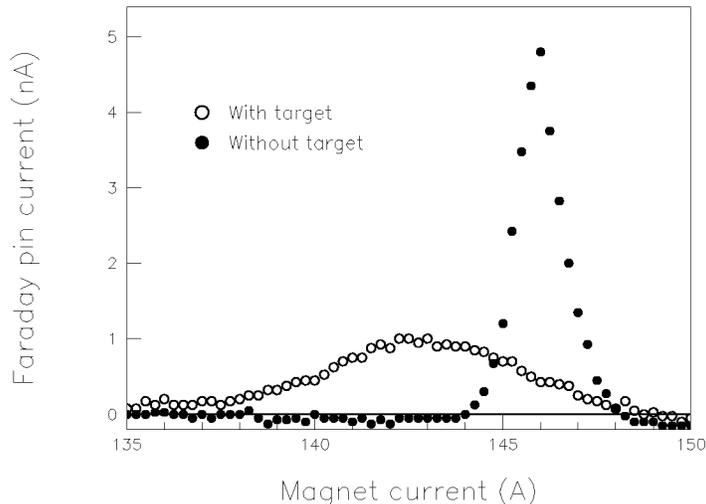
Figure 2: Example of a measured beam profile. The open and filled circles shows the profile with and without a lithium target, respectively.
