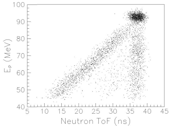
Figure 7: Proton energy versus neutron time-of-flight for  $(n,p)$  events, obtained using a  $\text{CH}_2$  target. Neutrons corresponding to the full-energy peak appear as a vertical band to the right.
