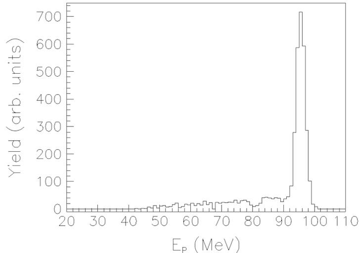
Figure 8: Proton energy spectrum for (n,p) reactions in hydrogen, induced by 96 MeV neutrons, in the angular range 6–7°. The spectrum has been obtained by subtracting a  $^{12}\text{C}(n,p)$  spectrum from a proton spectrum coming from  $\text{CH}_2$ , after normalization.
