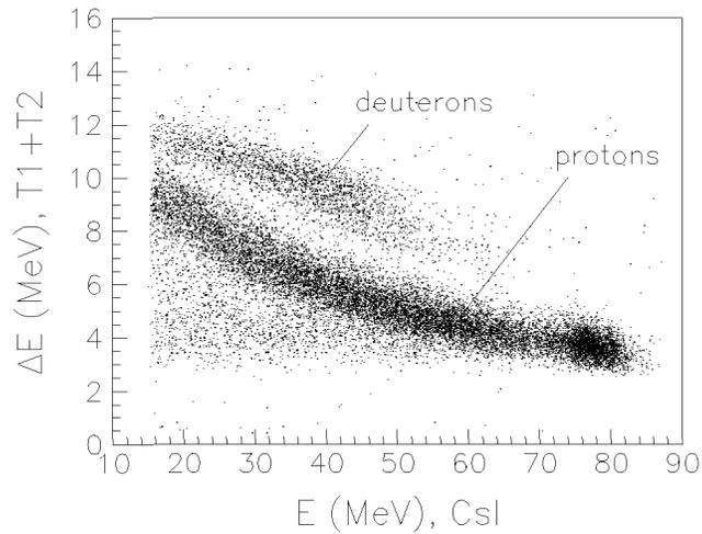
Figure 6: Two-dimensional scatter plot of the sum of the energies detected in the trigger scintillators versus the energy in a CsI detector at  $7^\circ$ . The data are obtained accepting protons from both carbon and  $\text{CH}_2$  planes in the multitarget.
