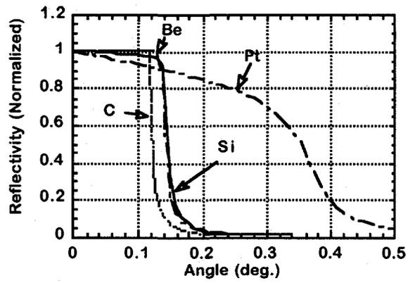
**Figure 1:** Reflectivity curves of Be, C, Si, and Pt at 1 Å radiation wavelength as a function of mirror angle.
