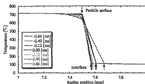
Fig. 12 Temperature distribution in steel particle, vapor film and liquid
