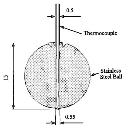
Fig.3 Structure of steel ball
