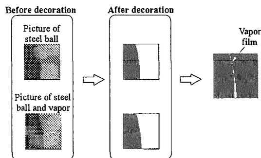
Fig.5 The determination procedure of vapor film thickness
