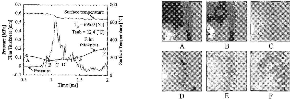
Fig.8 Surface temperature, pressure and film thickness in forced collapse experiment ( $T_{sub}=12.4^{\circ}C$ ).
