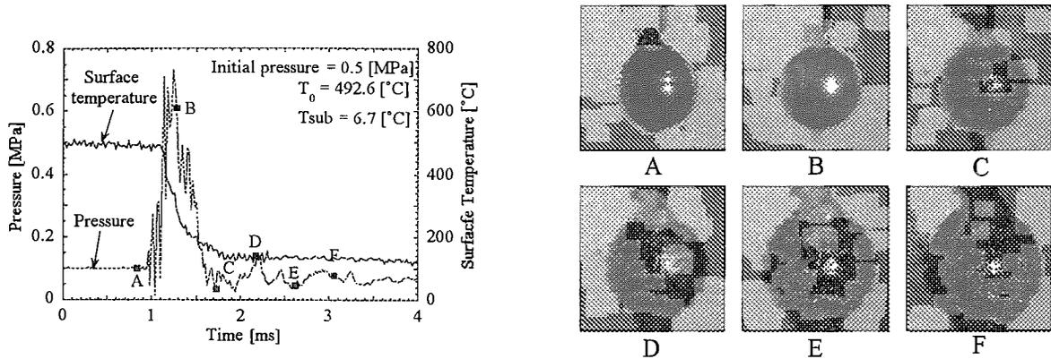
Fig.6 Surface temperature and pressure in forced collapse experiment
