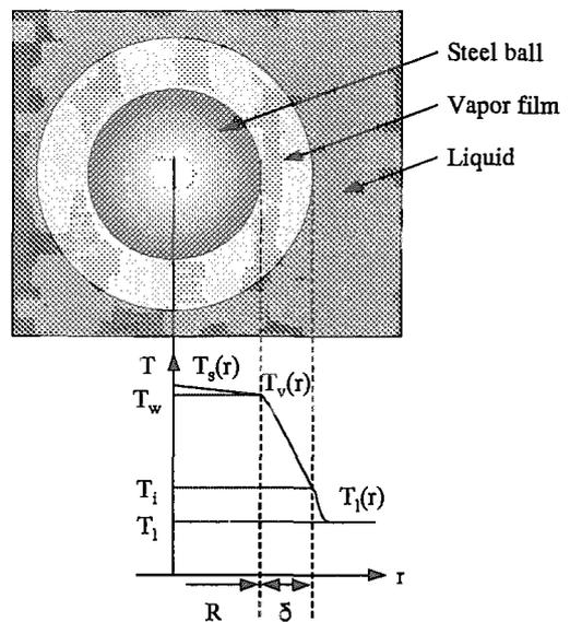
Fig. 10 Schematics of heat conduction analysis
