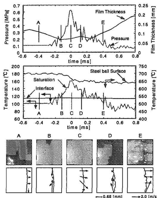
Fig. 19 Synthesis results from experiment and Analysis
