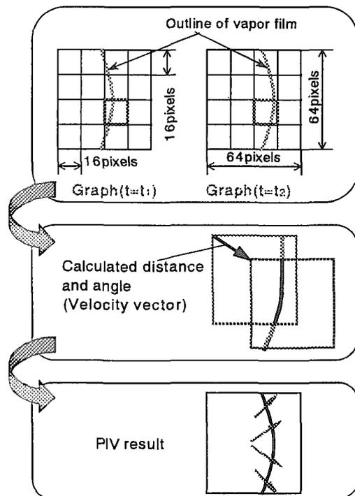
Fig. 17 Procedure of PIV analysis
