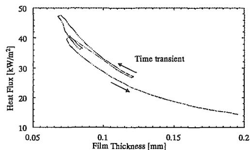
Fig. 14 Relationship between film thickness and heat flux at vapor-liquid interface
