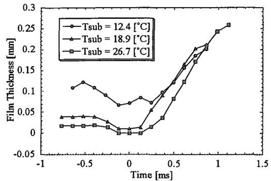
Fig.9 Time variation of film thickness in forced collapse experiment
