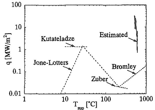
Fig. 15 Comparison with existing boiling curve
