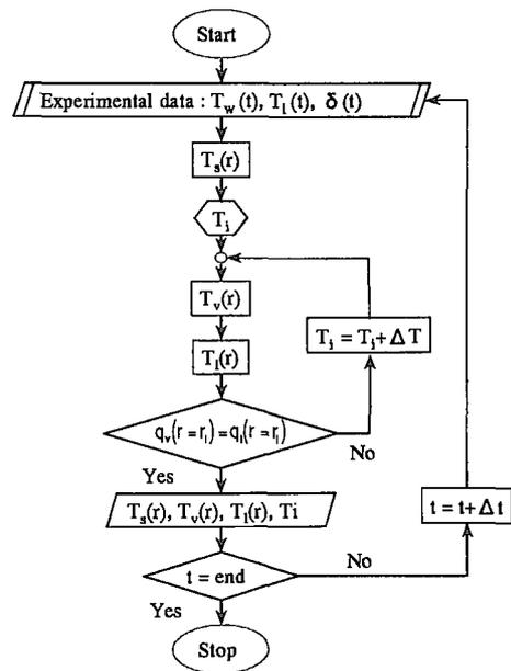
Fig. 11 Flowchart of heat conduction analysis
