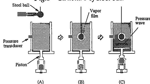
Fig. 4 Experimental procedure
