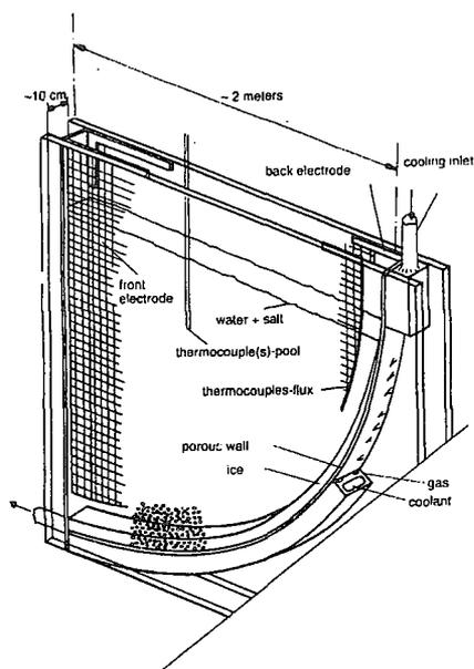
Fig. 2: Test facility of BALI
