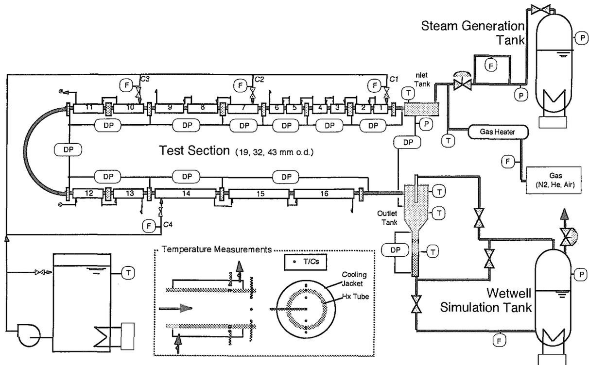
Fig. 4 Schematic of Test Facility for Fundamental Condensation Experiments
