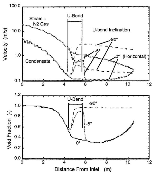
Fig. 6 Comparison of Calculated Fluid Velocities and Void Fractions for Different U-bend Inclinations (31.8 mm tube)
