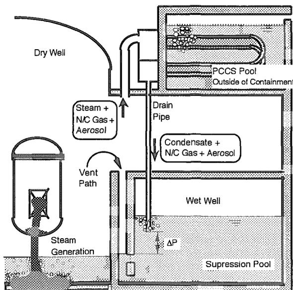
Fig. 1 Schematic of PCCS Operation
