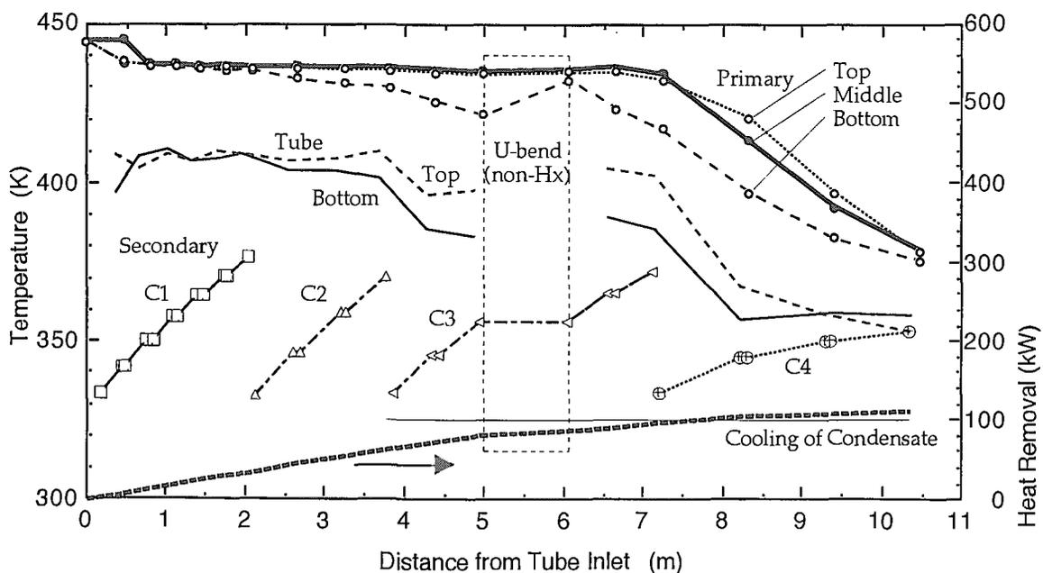
Fig. 5 Typical Temperature Data (Shakedown Test for 31.8 mm o.d. tube)
