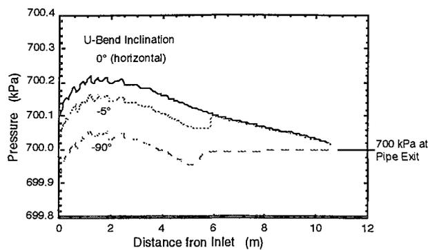
Fig. 7 Comparison of Calculated Static Pressures for Different U-bend Inclinations (31.8 mm tube)
