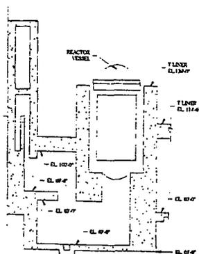
Figure 2-1 Section-view of Cavity
