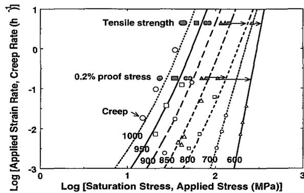
Fig. 4 Modeling of minimum creep rate given by modified Norton's Law for CF8M
