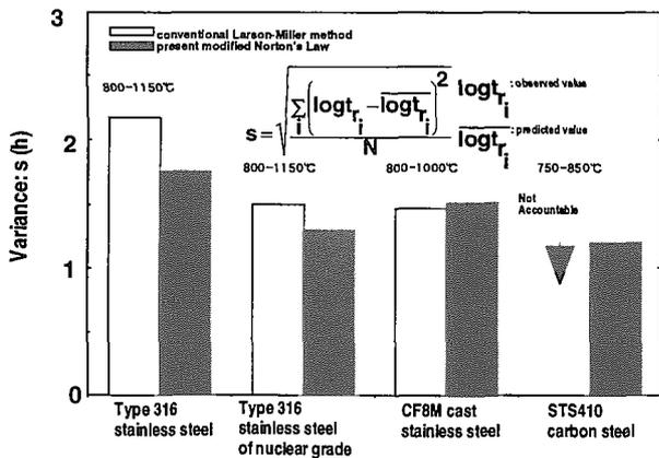
Fig. 3 Comparison of variance in model s of time to rupture for LWR piping materials
