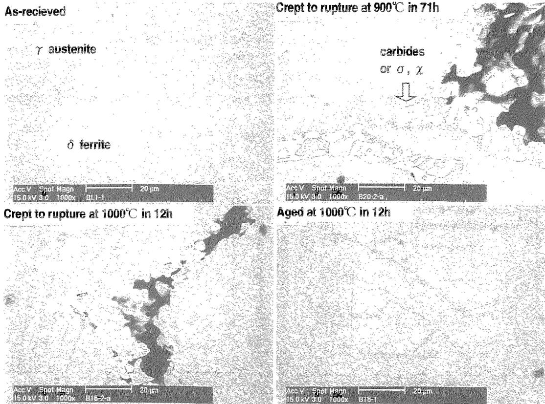
Photo.1 Microstructural change in CF8M duplex stainless steel at hot-temperature
