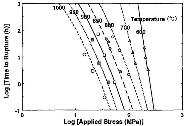
Fig. 2 Modeling of time to rupture given by modified Norton's Law for CF8M
