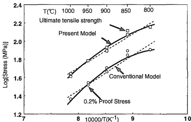
Fig. 1 Modeling of hot tensile strength for CF8M stainless steel
