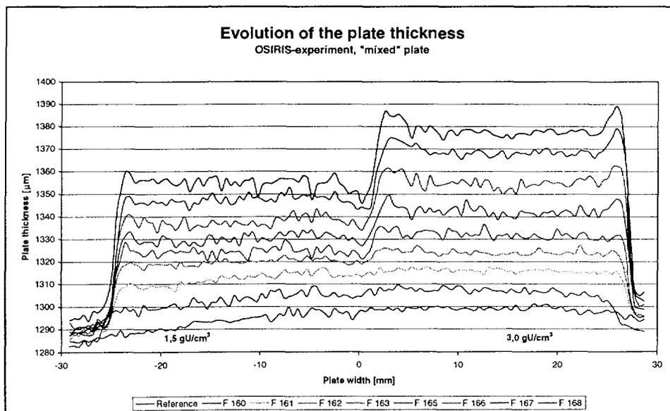
Figure 2: Measurements of the thickness of the mixed plate in transversal direction, i. e. perpendicular to the border between the areas containing fuel with an uranium density of  $1.5 \text{ gU/cm}^3$  and  $3.0 \text{ gU/cm}^3$ , respectively, available to date.
