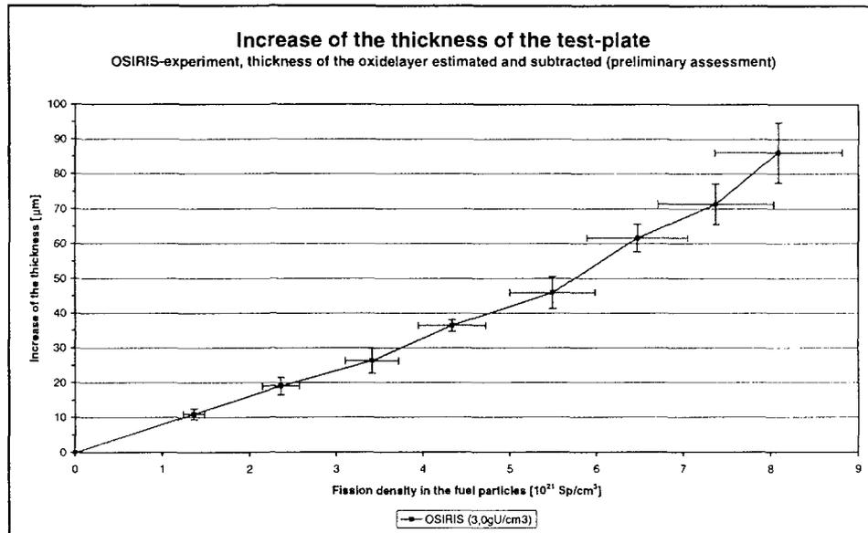
Figure 1: Increase of the thickness of the test-plate with an uranium density of  $3.0 \text{ gU/cm}^3$  as a function of the fission density in the fuel-particles. The thickness of the oxidelayer has been estimated and subtracted.
