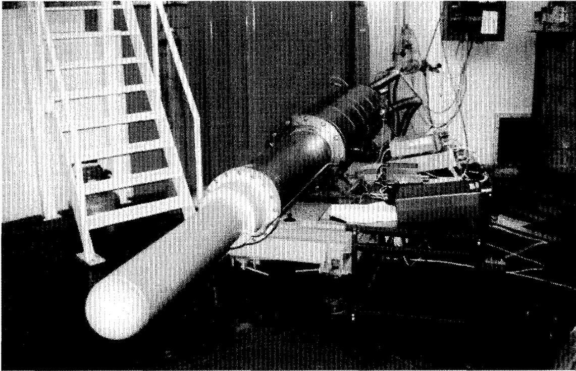
Fig 1. The cold plug in the time of out of reactor tests
