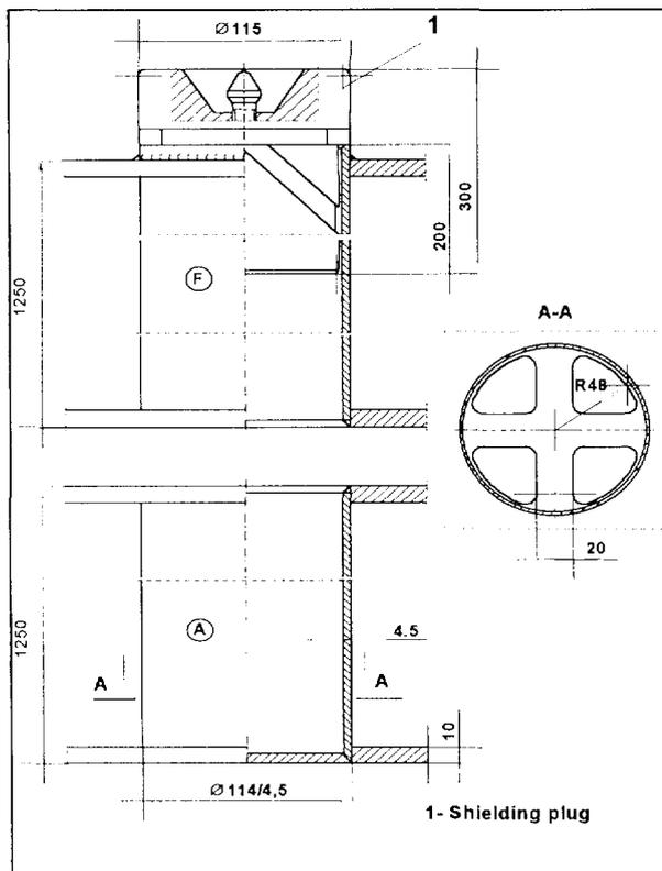
The storage channels of the separator (Fig. 3) are locked from the top by the shield plugs. Each of the plugs has a labyrinth channel for airflow, which enables the ventilation and cooling of the fuel providing simultaneously a shielding against radiation.
