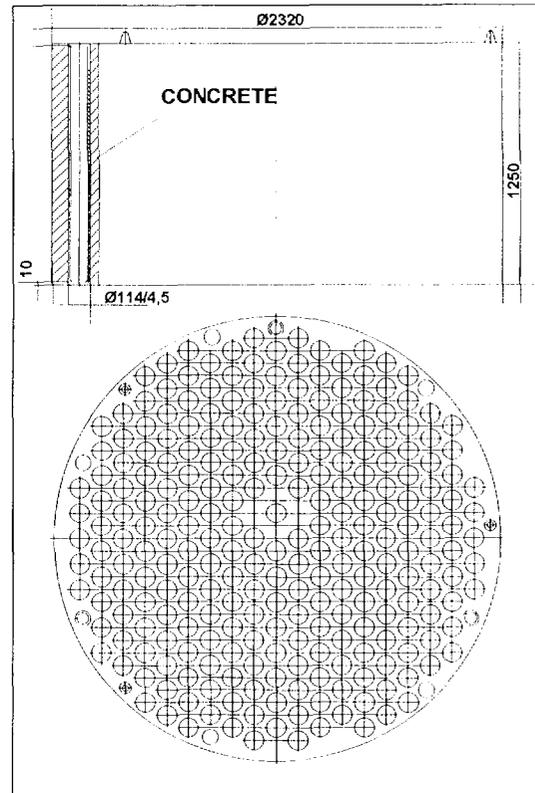
Fig. 2. Segment "A" of the separator
