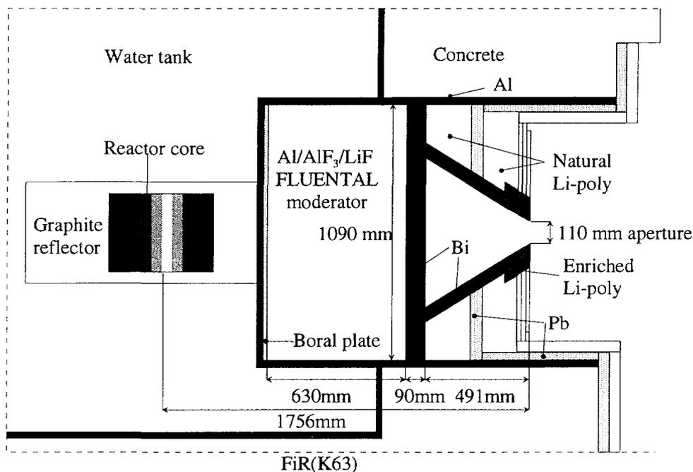
Fig 1. FiR 1 epithermal neutron beam facility
